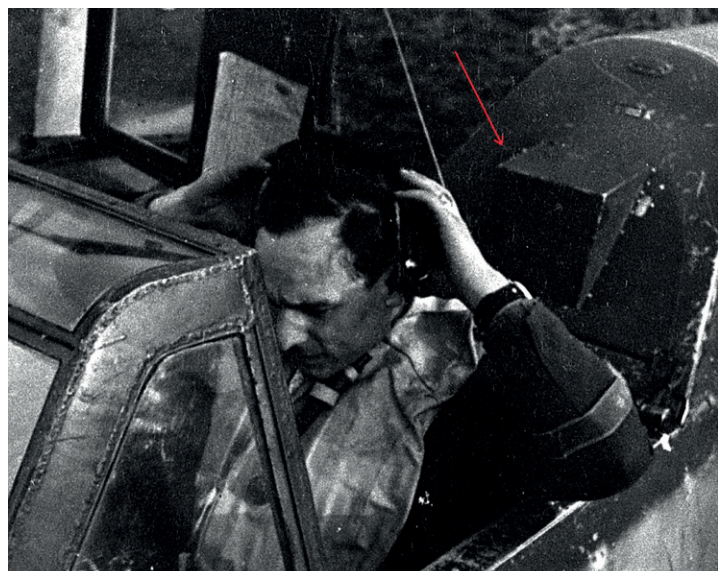
The protrusion on the access hatch to the battery and additional storage compartment allowed for the former's relocation forward, which freed up space for the MW 50 tank in the fuselage behind the cockpit. Bf 109G-14, Oblt. Rolf Schlegel 10./Jagdgeschwader 4, March 1945 [JG 4 Archive - Museum of the Air Battle over the Ore Mountains on September 11th, 1944 in Kovarska]
