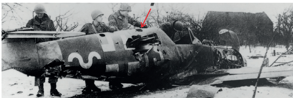
The wreckage of Bf 109G-10 WNr. 151556 from JG 300 and Bf 109G-14AS WNr. 784998 from IV/JG 53 after emergency landings in early 1945. Both aircraft show open MW 50 fuel tank filler ports on their spines.
