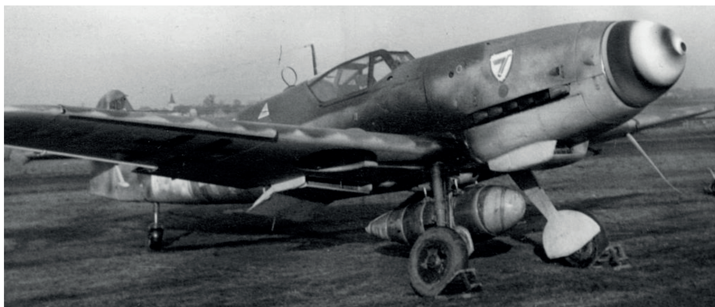
Bf 109 G-10 W.Nr 490 617 'Blue 2', Uffz. Gerhard Reiher, 8./JG 3, Alperstedt, 1944. Behind the circular antenna on the spine, a triangular label is visible adjacent to the MW 50 filling point [Martin Reiher]
