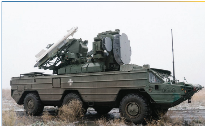
A Ukrainian modification of the old Soviet 9K33 Osa anti-aircraft system for the use of R-73 air-to-air missiles.
