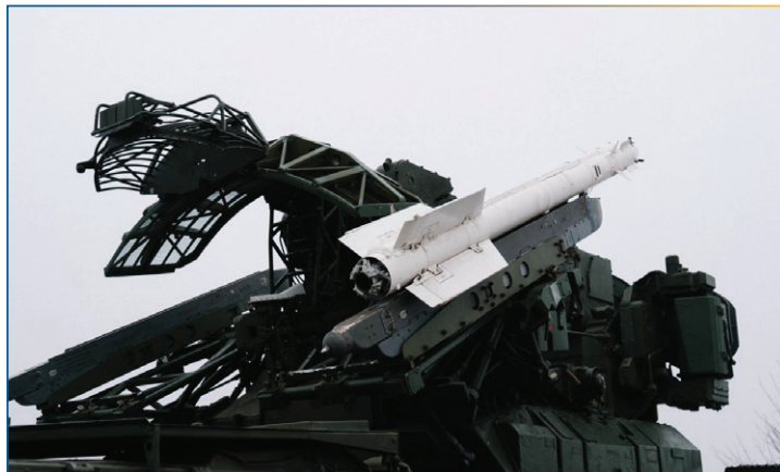
A Ukrainian modification of the old Soviet 9K33 Osa anti-aircraft system for the use of R-73 air-to-air missiles.
