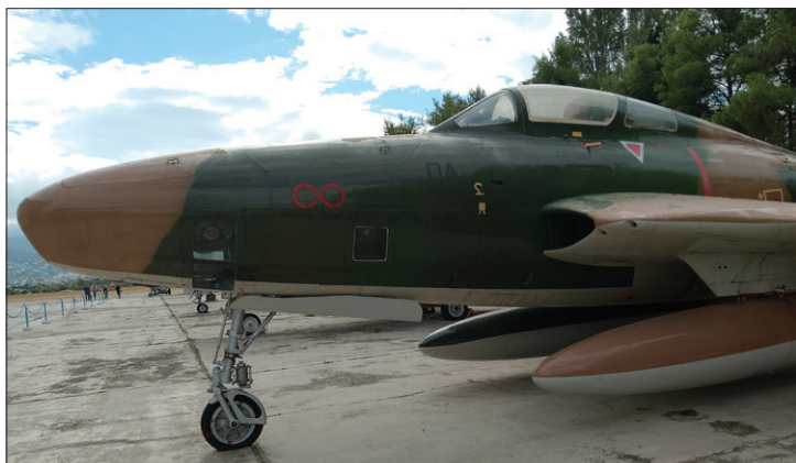
Bow section with cameras of the tactical reconnaissance Republic RF-84F Thunderflash
