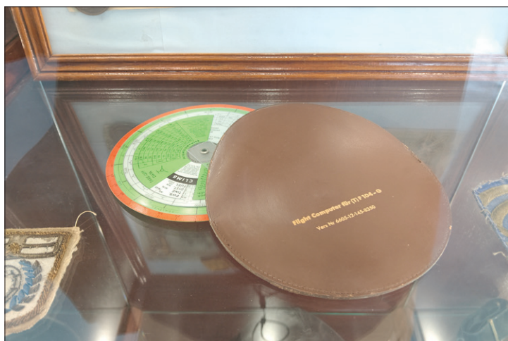
A mechanical computer for the F-104G pilot helped with flight time or fuel consumption data
