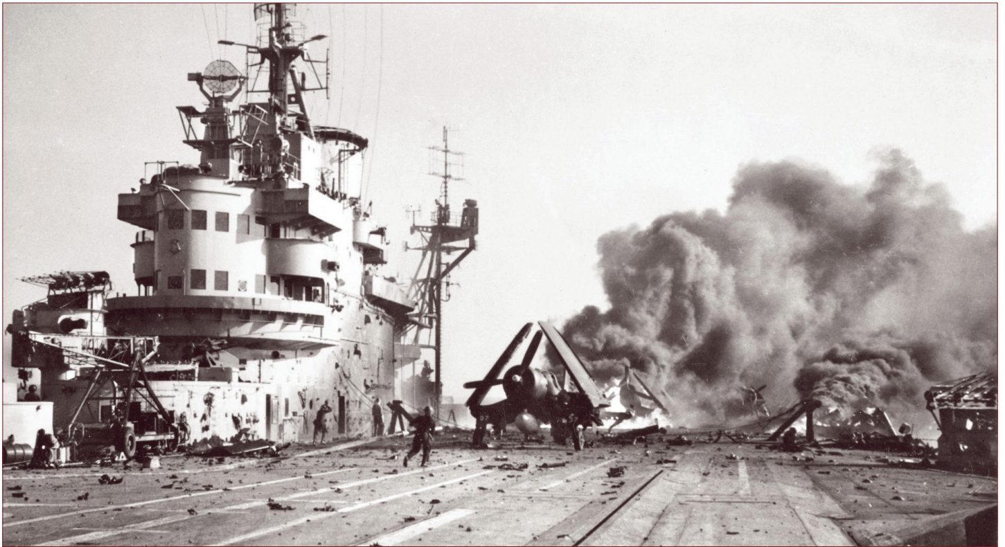
The British aircraft carrier HMS Formidable in May 1945 after a kamikaze attack. The armored decks of British aircraft carriers withstood enemy attacks much better than the decks of American carriers. Photo: IWM
