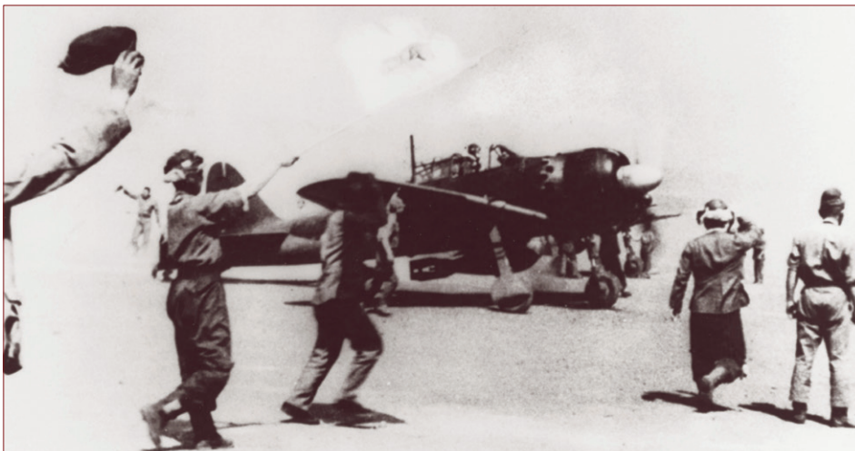
The A6M5 Type 52c aircraft taking off on a special attack mission. A 500kg bomb is mounted under the fuselage, and the cannons have been removed to reduce weight. Only two machine guns were left in the wings. Photo: US Naval Heritage Command
