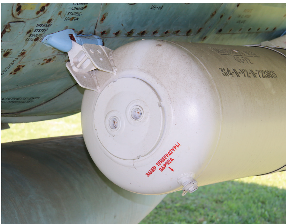
SPRD-99 RATO bottle, with the method of attaching the front mount and the shape of the bottle itself visible. Photo: Ing. Martin Janousek
