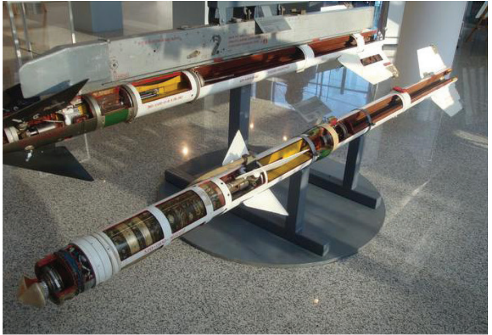
R-3R air-air guided missile in cross-section. Compared to the R-3S missile, the extended section housing the semi-active radar guidance electronics is clearly visible. In behind it is a cross-section of the R-13M missile mounted on its launch rail.
