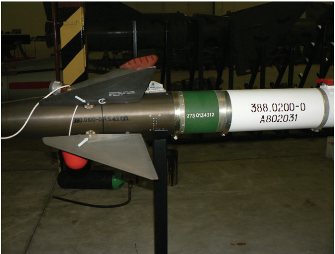
Warhead and proximity fuse, R-13M
