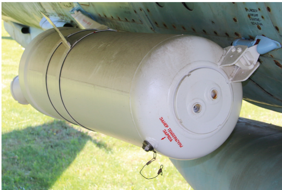
SPRD-99 RATO bottle, overall view of the installation method under the right side of the fuselage. Photo: Ing. Martin Janousek
