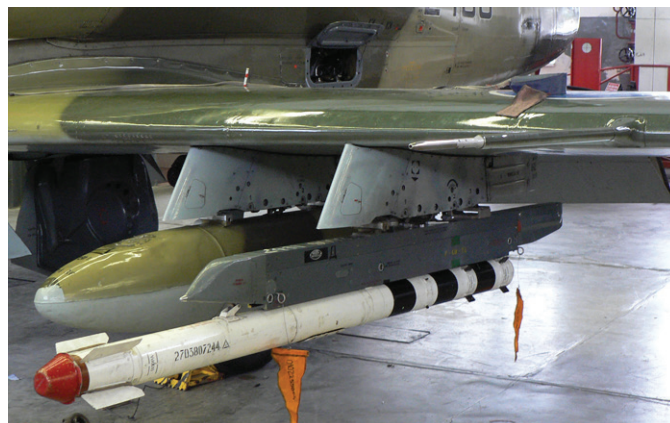
For training purposes, a UZR-60 acquisition round was developed (shown here slung under an L-39ZA Albatros), which was easily identifiable by the three black bands around the rear of the missile. The fins on this type of piece of equipment were removed, as was the rocket motor and warhead. An internal evaluation device that recorded certain data during target acquisition was installed in these rounds. Two arming pins are installed with RBF tags for visibility.
