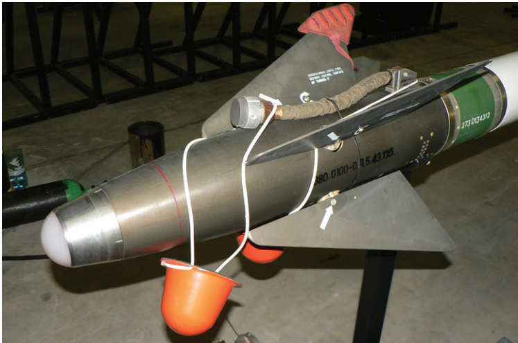
Guidance and Control Section of the missile. In the upper part of the control section, a pull-out cable connection is visible, which connects the missile with the aircraft's onboard network.
