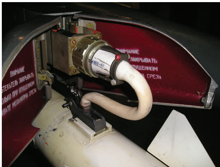
Open forward edge of the launch rail, into which the communication cable is connected, located in the missile's control section.
