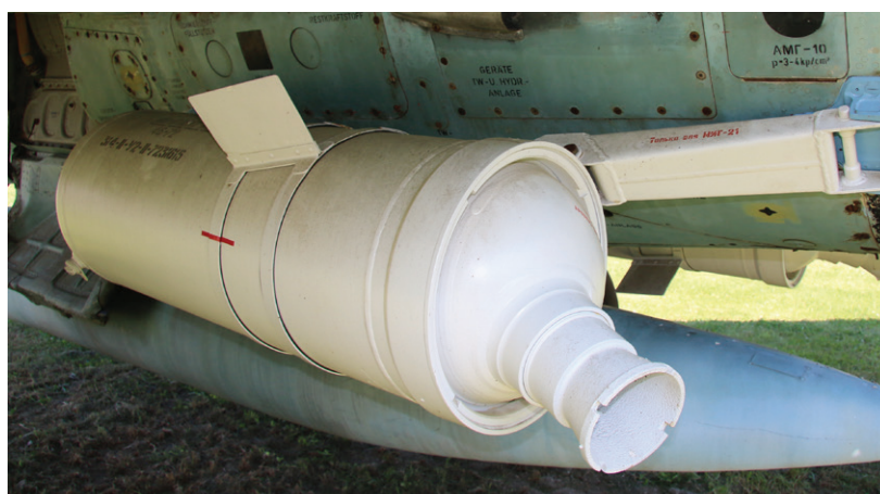
SPRD-99 RATO bottle installed under the left half of the fuselage of a MiG-21bis of the former GDR Air Force. The method of attaching the rear of the bottle and details of the nozzle are visible. Photo: Ing. Martin Janousek
