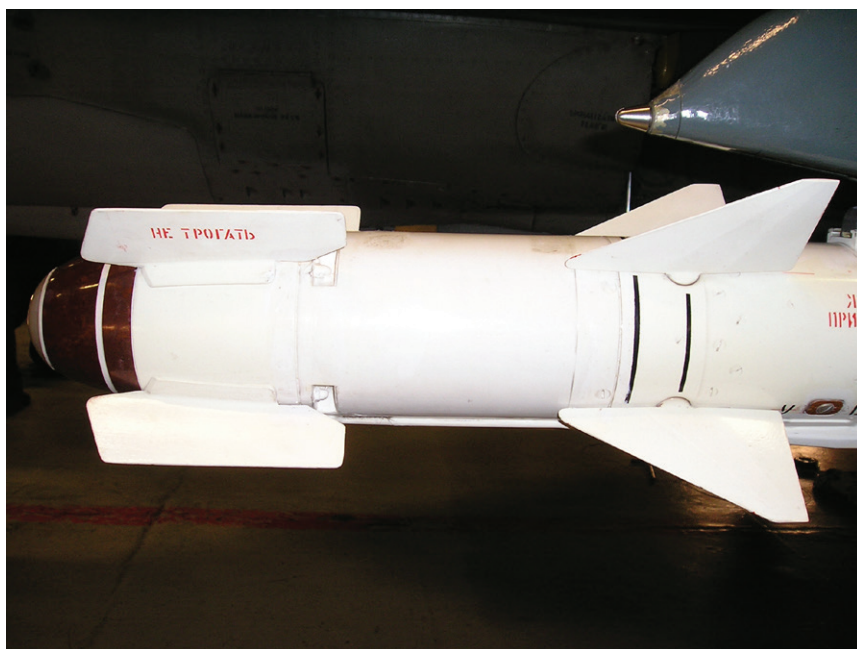
Infrared seeker head with destabilizers, to which is attached the warhead (between the destabilizers and rudders) of the R-60M missile.
