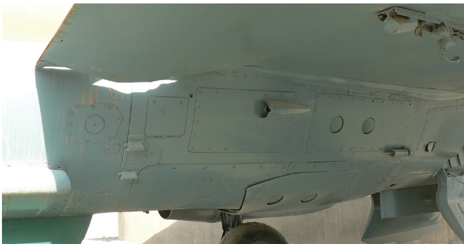
A detail shot of the same airplane showing the front and rear attachment points for the right SPRD-99 RATO bottle.
