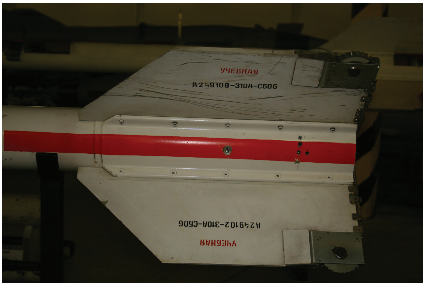
Stabilizing fins of the R-3S missile (note the red stripe and inscription). It is also worth noting the slightly different design of the rollerons compared to the more modern R-13M missile. The missile is suspended under and launched from an APU-13 launcher rail.
