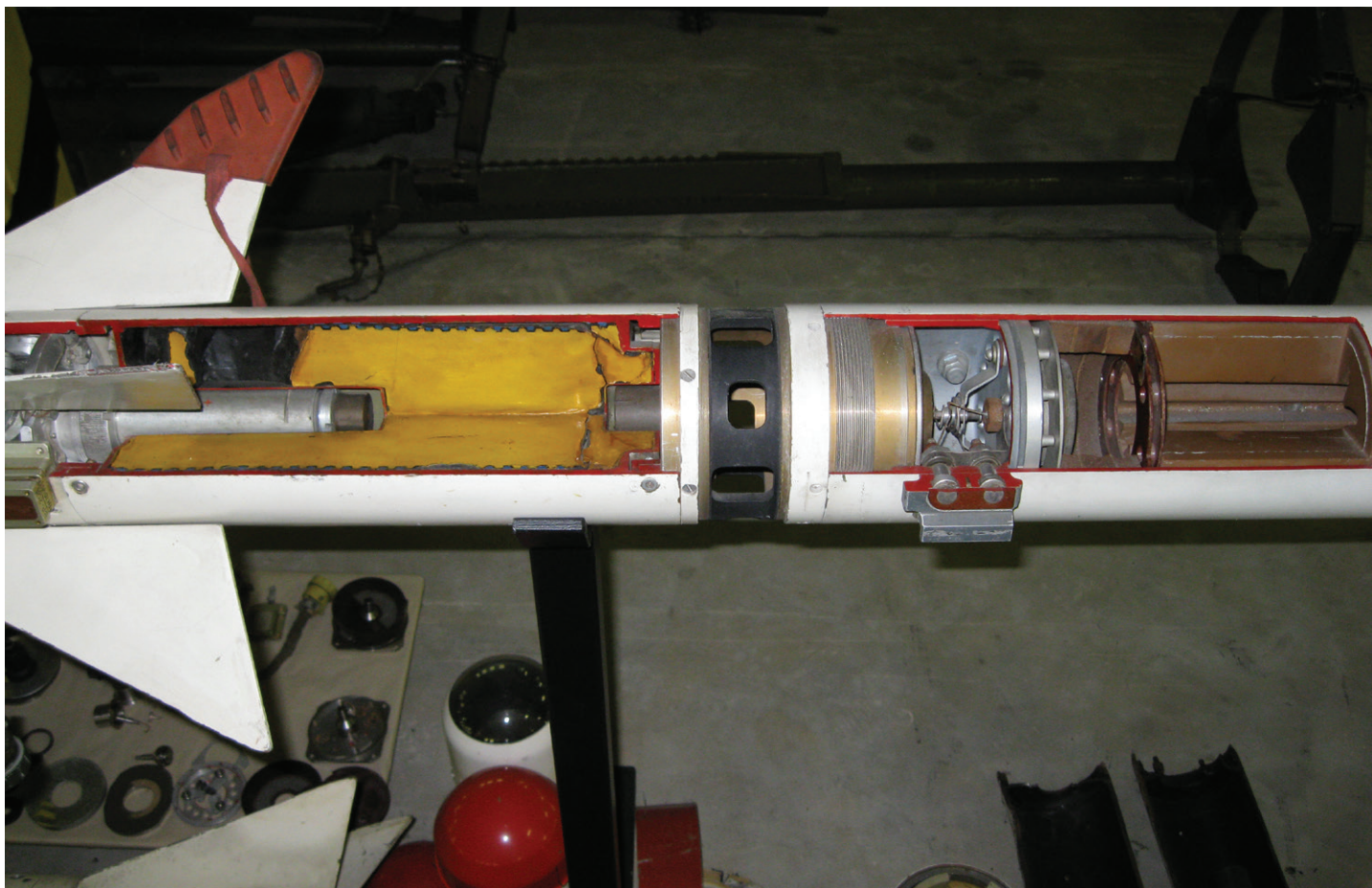
Proximity fuse and rocket motor of the R-3S in cross section.
