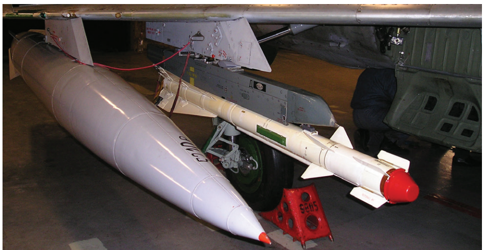
Overall view of an R-60M guided air-air missile with a red protective cap covering the seeker head, suspended from a simple P-62-IMD launch rail under a MiG-21MF.
