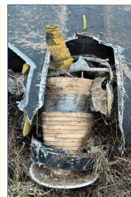
A "warhead" made of wooden slats inside a drone sent as a decoy to overwhelm Ukrainian air defenses.
