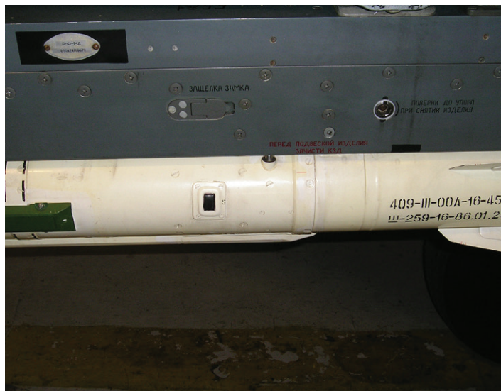
Power section, on the outer part of which are located the green antennas of the proximity detonator system and the R-60M launch indicator.
