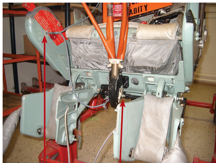
Lock numbers 1 and 2 locations on the KM-1M seat
