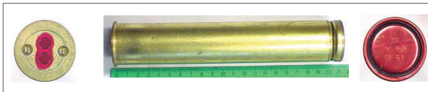
PK-16M from the left, a bottom view with two fuses, side view, and cover with stencil data
