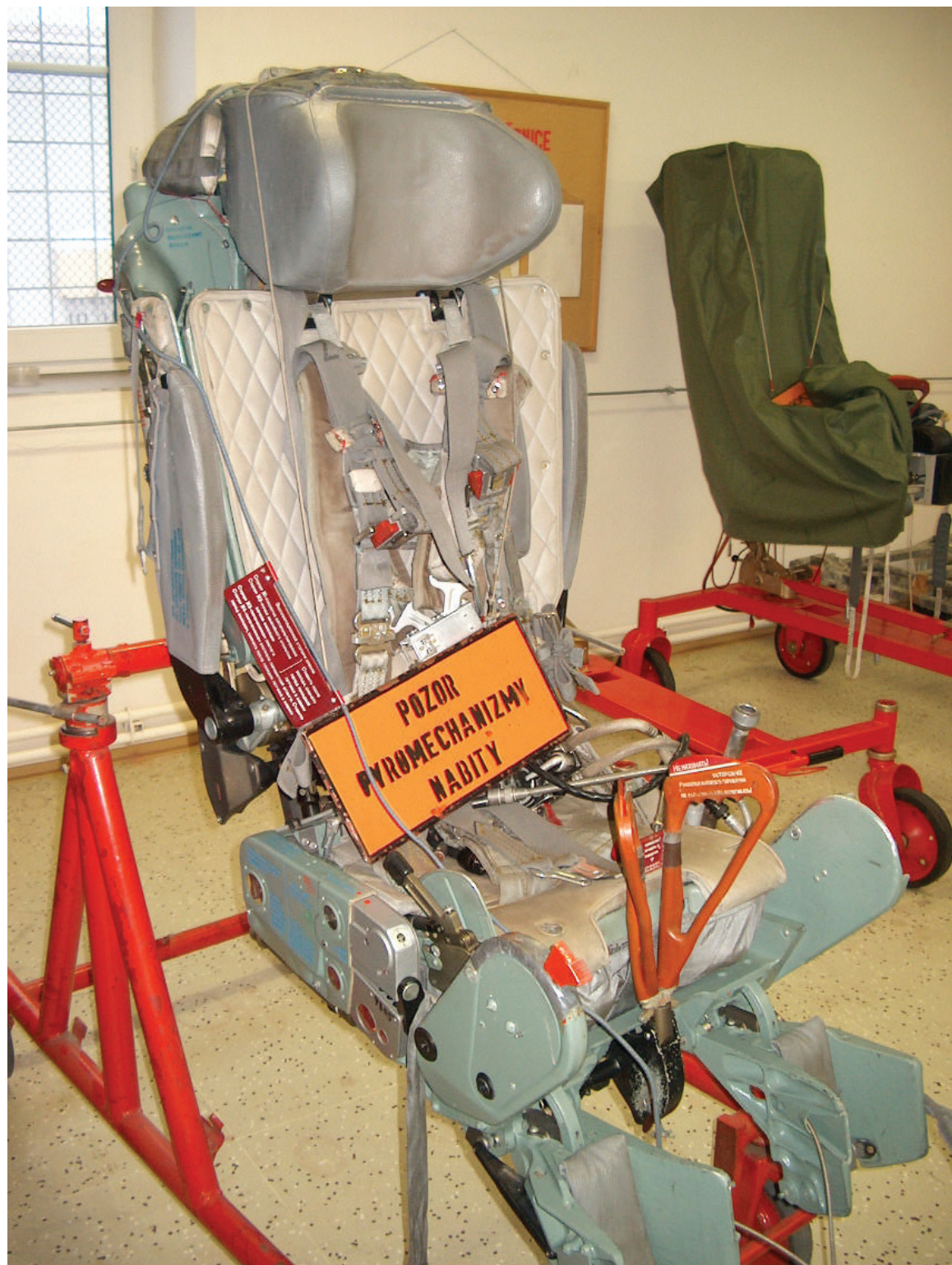
Overall view of the KM-1M ejection seat removed from the aircraft for maintenance with the orange warning sign indicating that the seat is armed with explosive devices.
