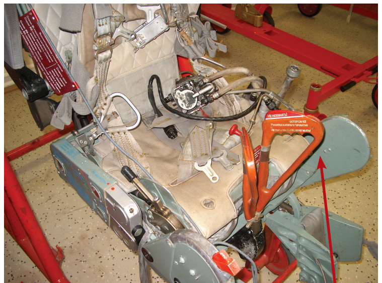
The ejection seat handles attached to the seat pan.
