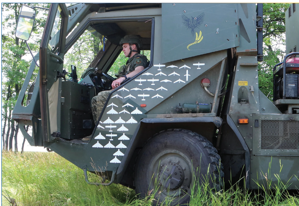
Raven is a cheap short-range mobile air defense system developed for Ukraine by the UK. It uses ASRAAM missiles on launch rails from decommissioned aircraft such as Jaguar and Tornado. The chassis is a Supacat HMZ 600. As the photo shows, Raven has proven itself in Ukraine.
