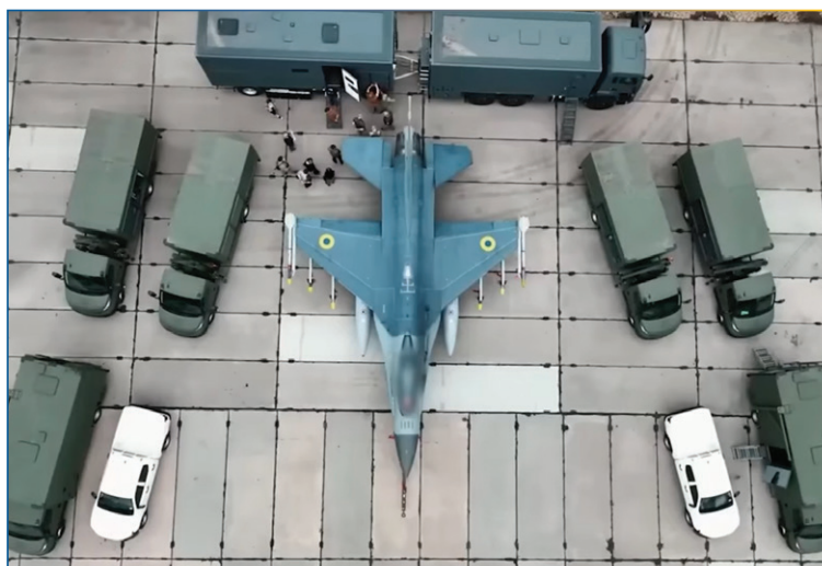
A Ukrainian F-16 fighter and the mobile complex that assists with aircraft maintenance during relocations between airfields.
