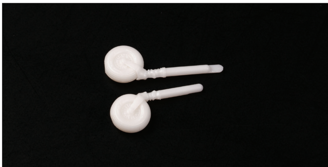
There are two types of tail wheel leg: short and long.
