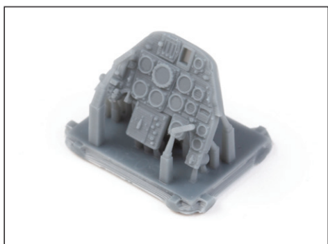
Thanks to 3D printing, the instrument panel, including the levers, is made from a single piece. These levers could not be moulded from plastic; in a conventional model, they would only be represented by a tiny etched part. Using them is problematic for many modellers anyway.
