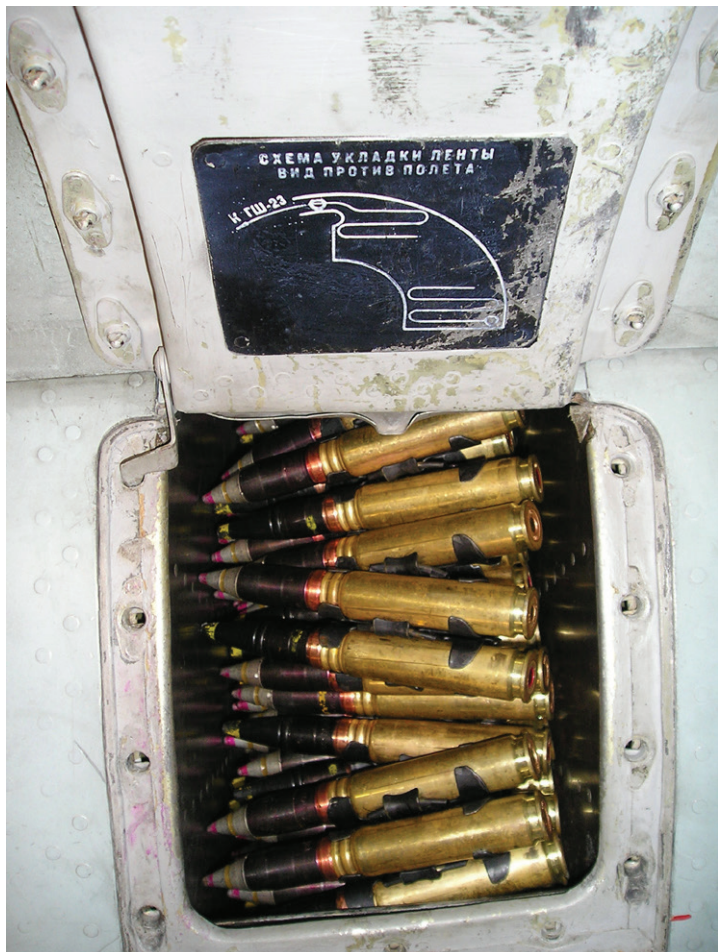
Ammunition box with a belt of 23 HE and 23 APIL ammunition in a MiG-21MFN, on the lid of the cover there is a diagram of the storage of the ammunition belt in the fuselage of the aircraft which contained a maximum of 200 rounds.
