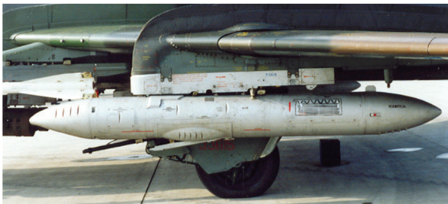
SPPU - 22 - 01 containers were originally developed for Su-17M3/M4 fighter-bombers (export variant Su-22M3/M4), and were later extended to MiG-27K/M/D series aircraft and Su-25 attack aircraft. The photo shows an SPPU - 22 - 01 on a Su-22M4 aircraft.
