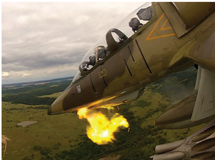
The GSh-23 aircraft cannon in action, firing from an Aero L-39ZA Albatros aircraft, coded 3903 from the 222nd Training Squadron, the 22nd Air Force base in Náměšť nad Oslavou. The cartridges, which are ejected from the aircraft after firing and fall freely to the ground, as well as the luminous tracer rounds, are worth noting.
