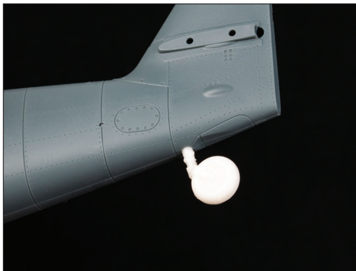
There are two types of tail wheel leg: short and long.
