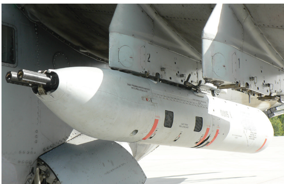
GSh-23L aircraft cannon in a UPK-23-250 pod. With pre-flight preparation completed, the cannon is ready to fulfill its training role at the aircraft shooting range.
