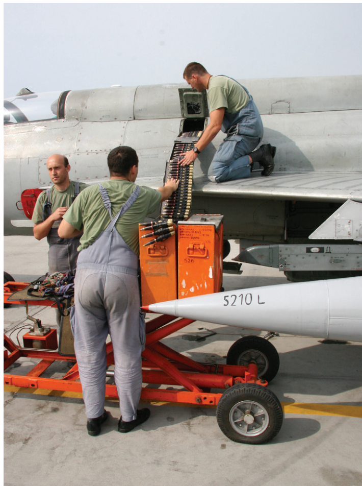
A pair of armaments specialists reload the full capacity of 200 rounds of ammunition into a MiG-21MF aircraft under the watchful eye of their armor crew chief.
