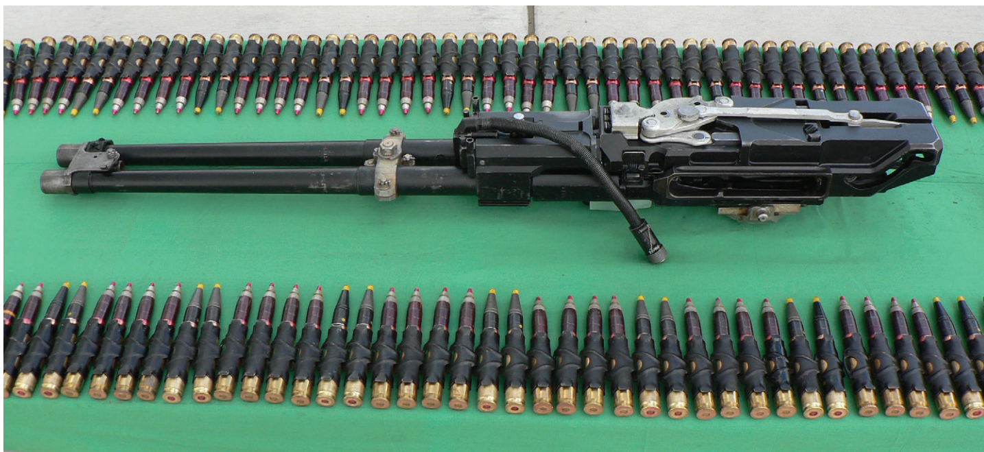
A GSh-23 unit attached to an Aero L-39ZA Albatros with 150 round capacity.
