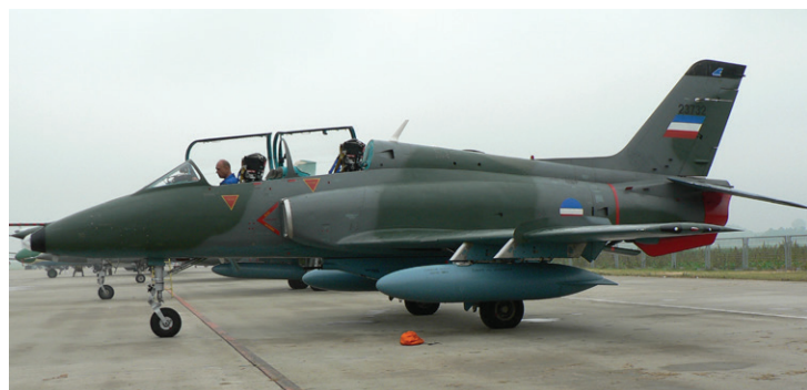
Serbian G-4 Super Galeb trainer aircraft with a GSh-23L cannon under the fuselage, in line with the rear cockpit.
