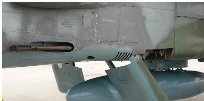
Detail of the GSh-23L cannon on the left, lower side of the NJ-22 Orao fuselage, in line with the engine intake.
