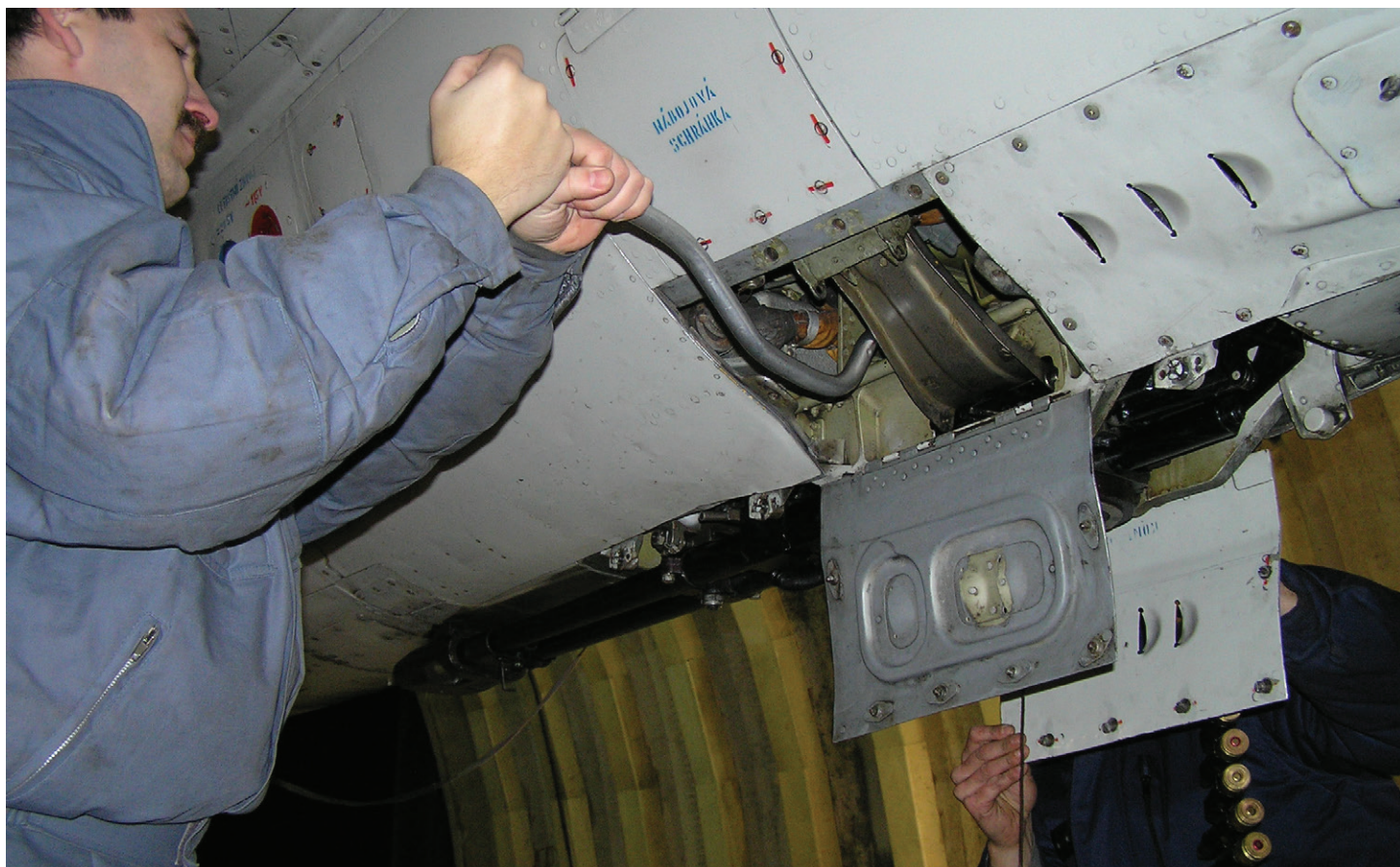
Preparing the GSh-23 cannon of a MiG-21MF deployed on a quick reaction standby. It is worth noting the special shape of the cocking lever in the armor's hand on the left and the uncovered cannon compartment for easier maintenance and handling.
