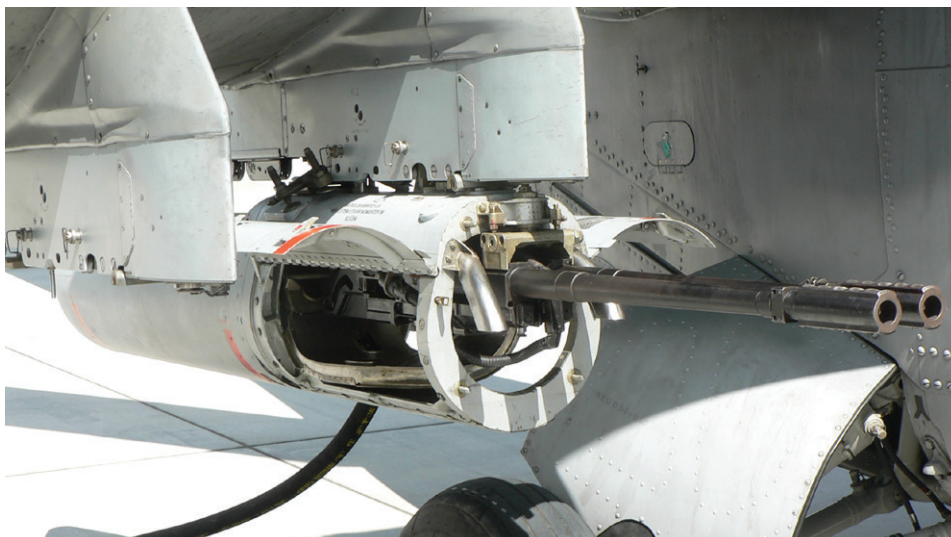
GSh-23L aircraft cannon mounted in a UPK-23-250 universal cannon container on a Mil Mi-24V attack helicopter. The front aerodynamic cowling is dismantled for pre-flight inspection and is carried out in association with charging the unit for live fire operation.
