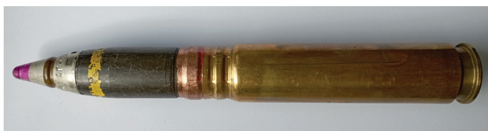
HE round with AG-23 fuse with copper remover (different manufacturer; gray bullet body and a yellow copper remover marking strip located in the upper part of the round).
