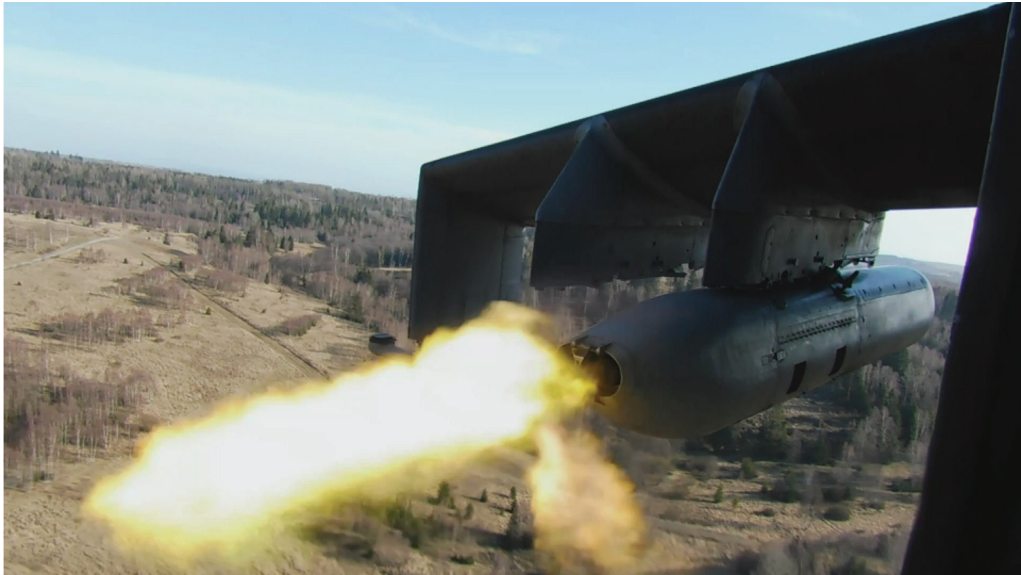
The GSh-23L cannon in action while firing from a UPK-23-250 container on a Mi-24V helicopter.
