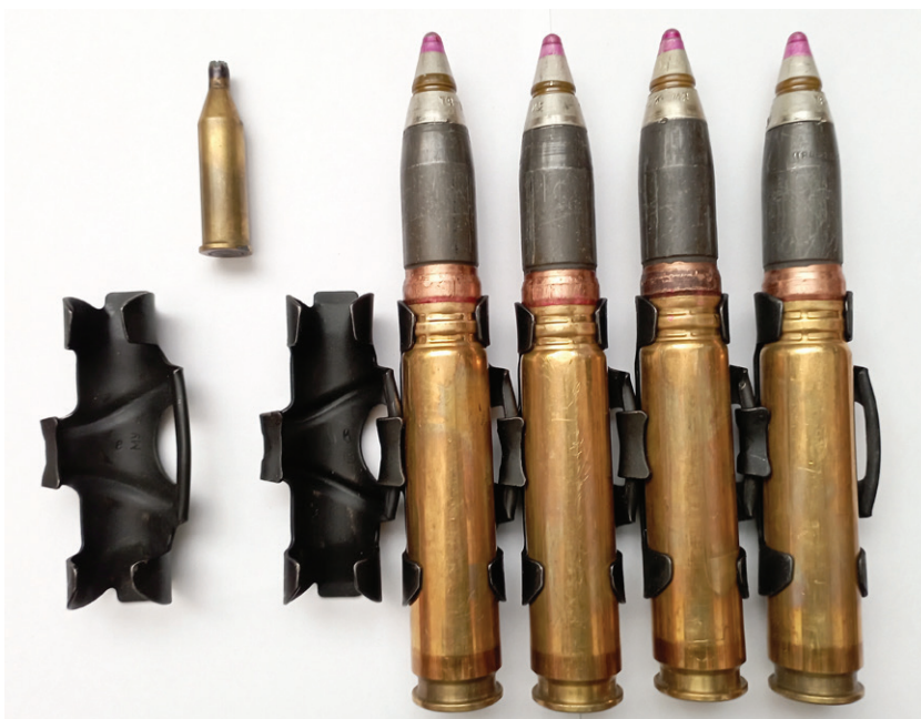
Ammunition belt section consisting of four rounds of 23 OFZ and fragmentation rounds. For comparison, in the upper left corner is a PPL pyro cartridge, used to cock the weapon before firing.
