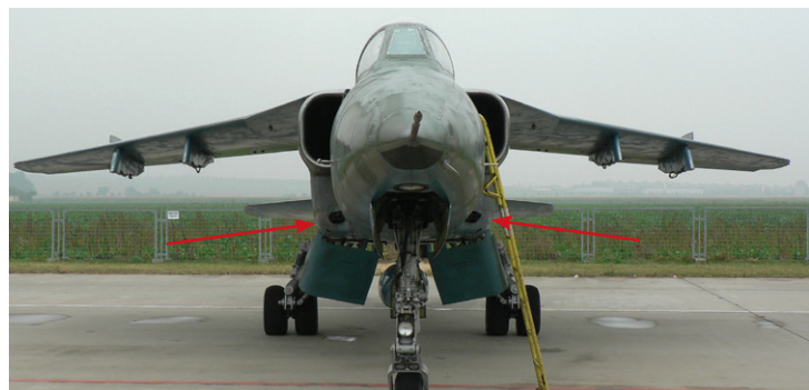
Serbian NJ-22 Orao training and light attack aircraft in front view. The weapons are installed in the lower part of the fuselage, indicated by the arrows.
