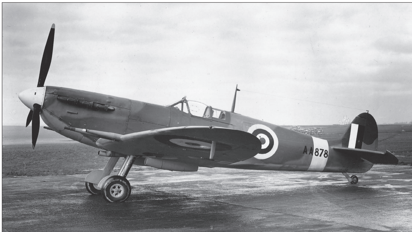
Spitfire Mk.Vc armed with four Hispano Mk.II cannons. Propeller is De Havilland, new canopy style with interior glass armor on the windshield and bulged sides of the canopy sliding portion. The aircraft supposedly carries an older type of radio Tr.9D (photo: Simon Erland).
