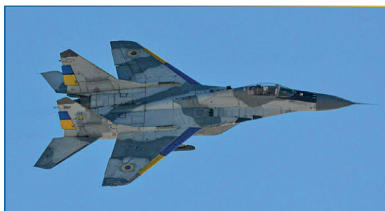
New images of the ex-Slovak MiG-29AS fighters. The characteristic antenna behind the cockpit, overpainted original markings, and heavily worn paint can be noticed.
