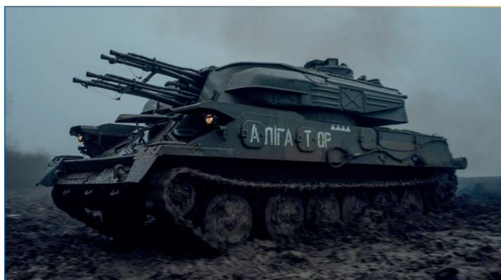
Soviet ZSU-23-4 Shilka systems, recently modernized by Ukraine, are also being used against drones. This vehicle was named "Aligator" and sports four kill markings.
