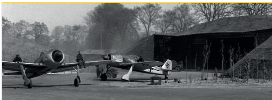
This photograph of aircraft from II./JG 26 clearly shows the practice of carrying mechanics on the wing of the Fw 190, helping the pilot to orient himself while taxiing. Interestingly, the aircraft on the left is an Fw 190 A-1, that is, fitted with 7.92 mm machine guns in the wing roots. II./JG 26 used this early Focke-Wulf version until August 1942, alongside Fw 190 A-2 and A-3 aircraft. Photo: Bernie Thorsch Collection via Peter Merlin
