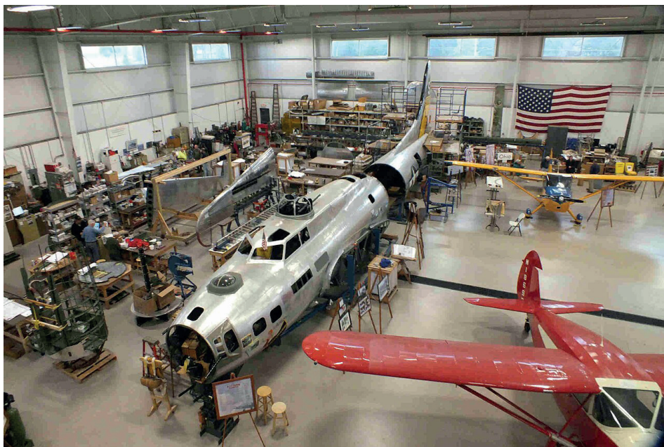
The B-17G, named 'Champaign Lady' after its place of origin, is assembled from the wreckage of at least five other Flying Fortresses.
