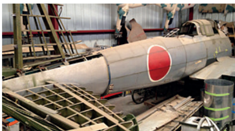
Restored tail surfaces of the Aichi D3A2 Type 99 (Val).
