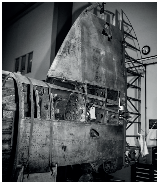
Original condition of the tail surfaces of Typhoon RB396.
