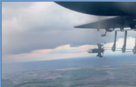
Launch of a P1-SUN interceptor from a hardpoint under the wing of an Antonov An-28.
