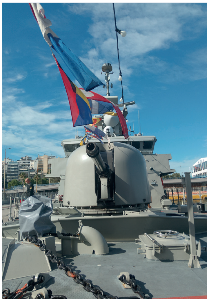
OTO Melara 76 mm naval gun mounted on the bow of the missile boat Karathanasis.
