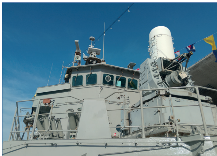
View of the forward superstructure and bridge of the frigate Psara. In the foreground is the Mk 15 Phalanx close-in weapon system equipped with a 20 mm Vulcan rotary cannon.
