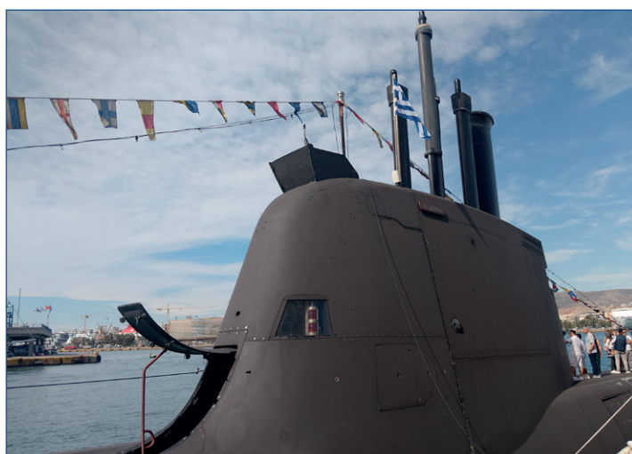
The sail of the submarine Pipinos. Its streamlined shape is particularly noteworthy. The open passage leads to the aft deck, as the sail's design makes it impossible to pass around it externally. It is therefore not an entrance to the pressure hull.
