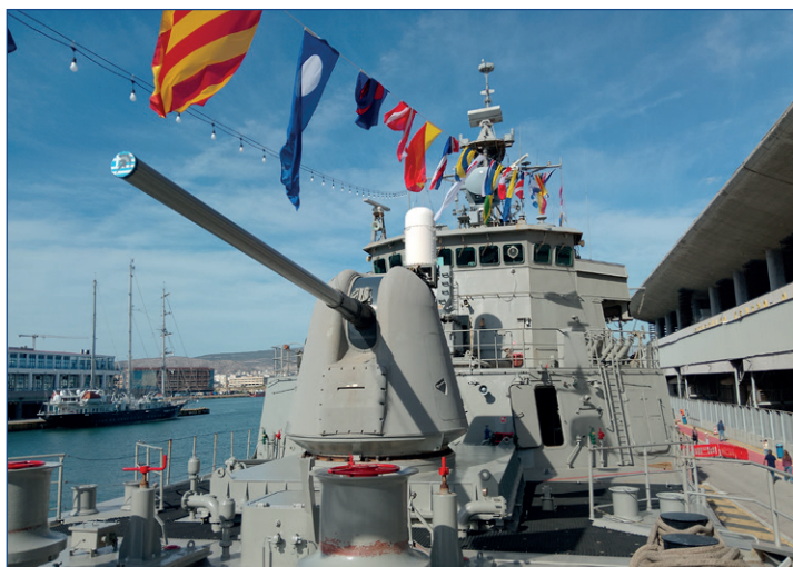
Mk 45 127 mm naval gun mounted on the bow of the frigate Psara.
