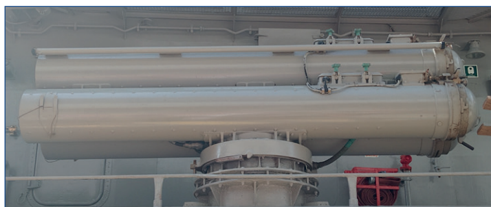
Mk 32 triple 324 mm torpedo launchers on the port side of the frigate Psara (F454).
