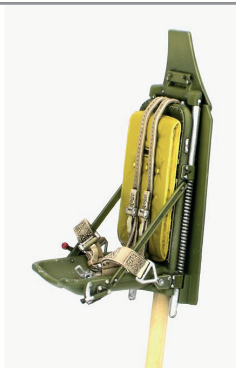
Pilot seat. On the left is a render, on the right is a painted model built from the kit. The kit includes two alternative seat designs. Like the seat itself, the seat belts are printed as separate 3D printed parts.
