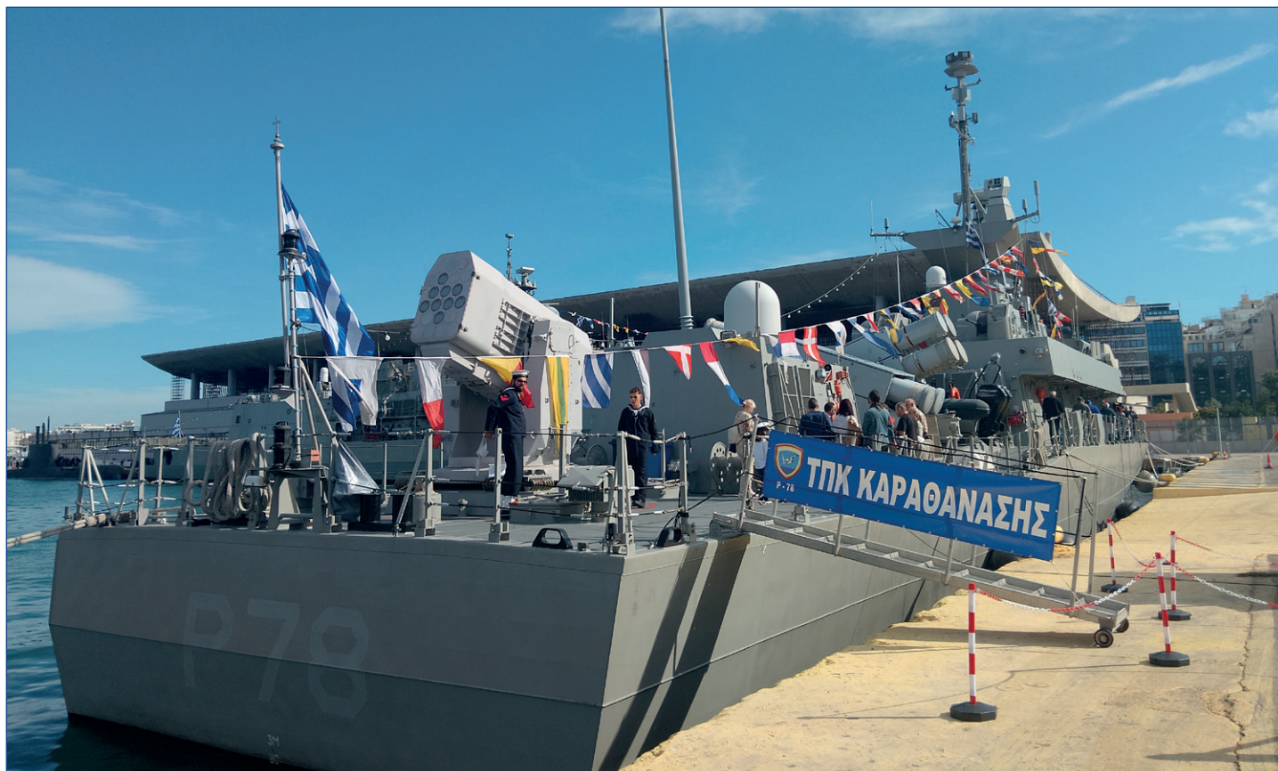
The stern of the missile boat Karathanasis (P78), with the short-range RIM-116 surface-to-air missile launcher.
