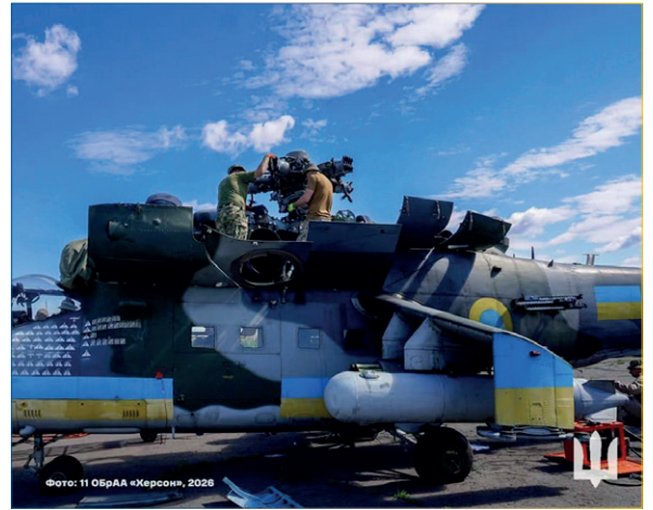
A former Czech Mi-24 helicopter undergoing an engine overhaul.
