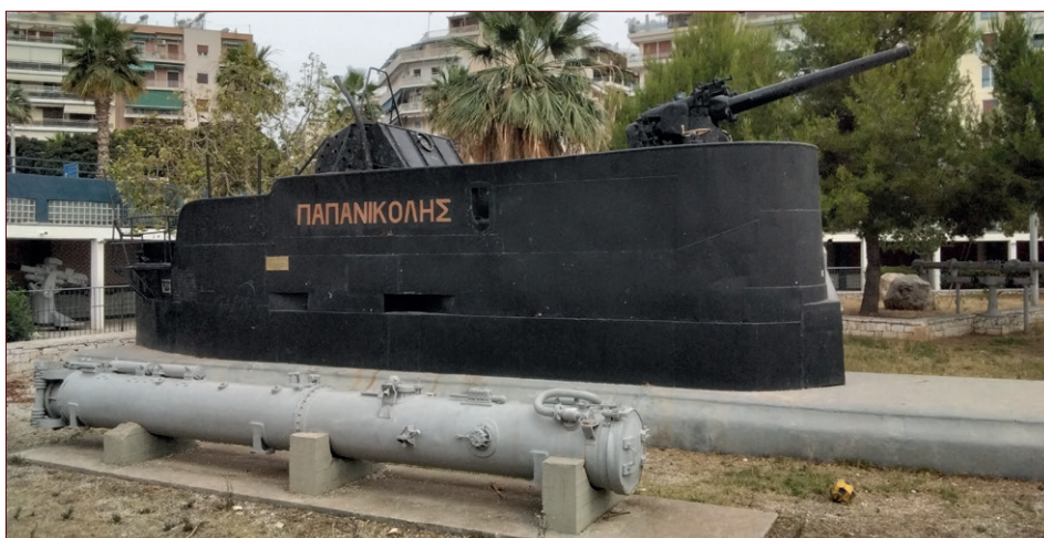
Side view of the conning tower of the submarine Papanikolis. Note the 100 mm deck gun and the preserved torpedo tube in the foreground.
