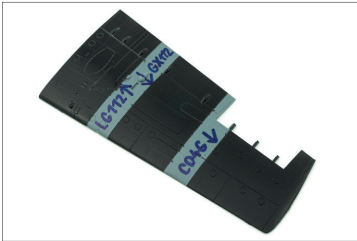
The test of gloss coats photographed in a softbox optically reduces the differences between the individual varnishes. This proves that the test results cannot be divided into good varnish vs. bad varnish, but under extreme lighting in the previous shots, the differences in the results, which are less noticeable in indirect light, can be seen better.
