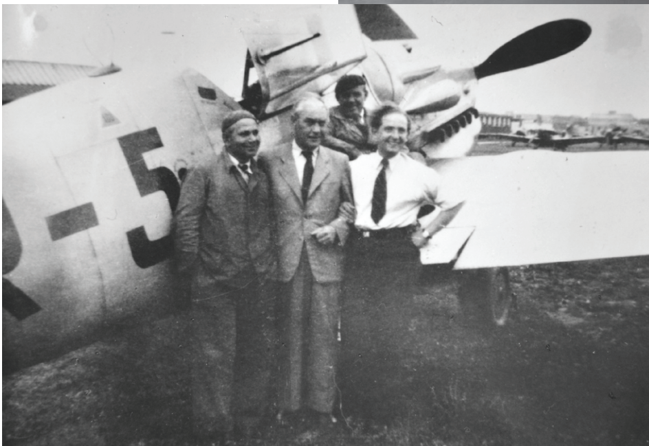
Rather poor quality but interesting photograph captures the aircraft of the staff flight of the 3rd Air Division marked IR-5 with number shaped in an unusual manner. This S-199 could not be identified further but is painted light green-gray overall and features the older type of "Erla Haube" canopy opening to the side.
