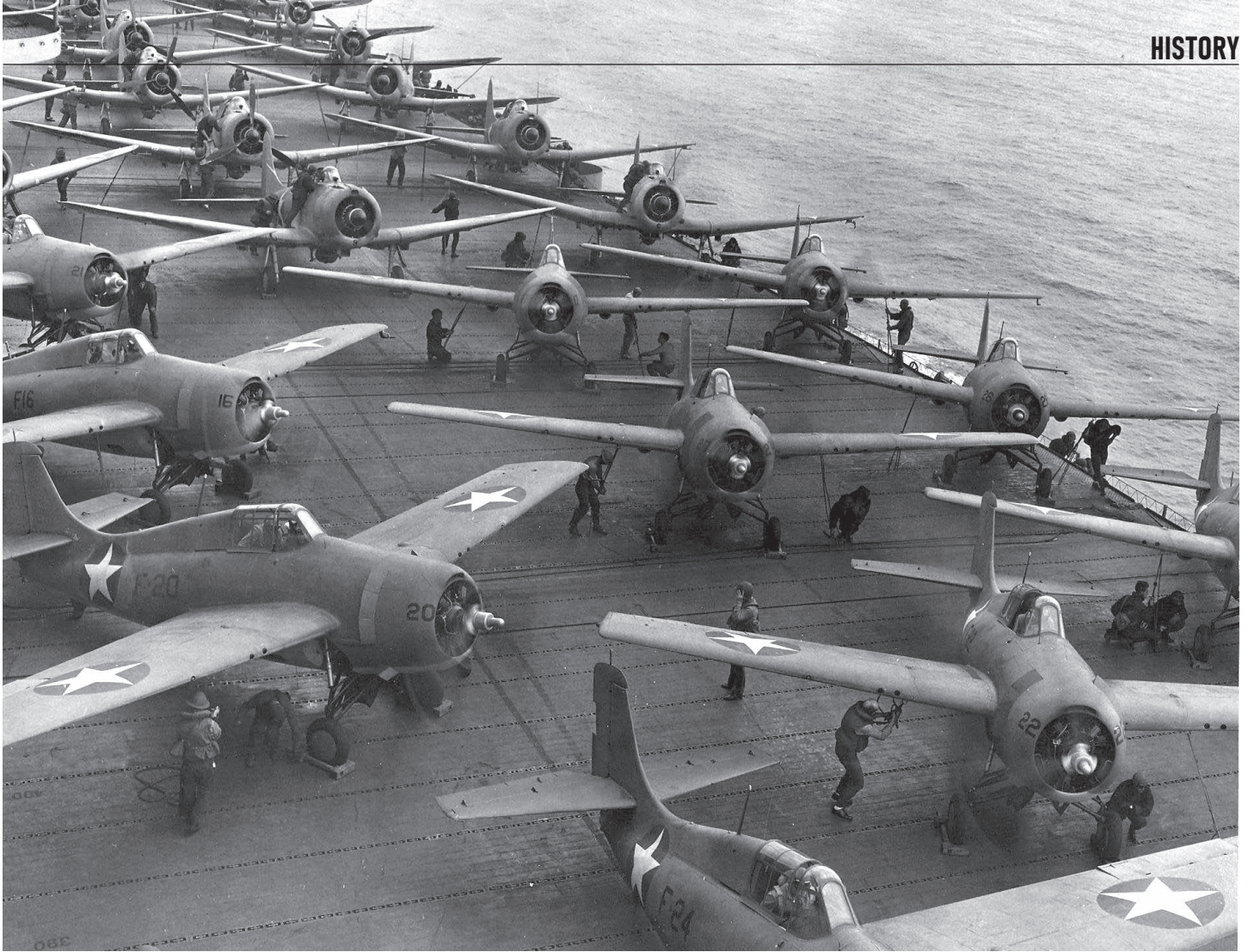
Adding wing-folding to the F4F-4 allowed the number of Wildcats aboard a fleet carrier to be increased by 50% over the non-folding F4F-3. (USN)
