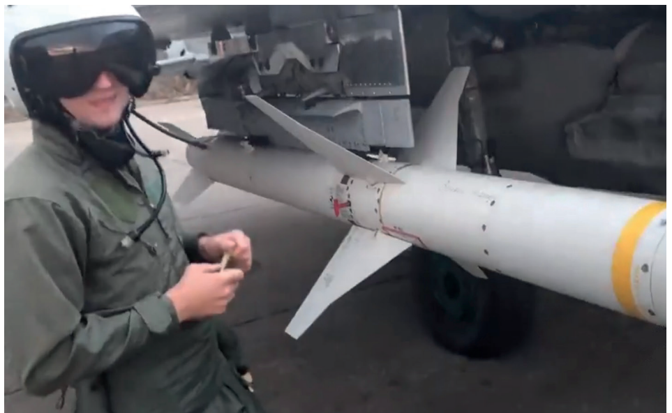
Detail of HARM missile fitted to the Ukrainian MiG-29.
