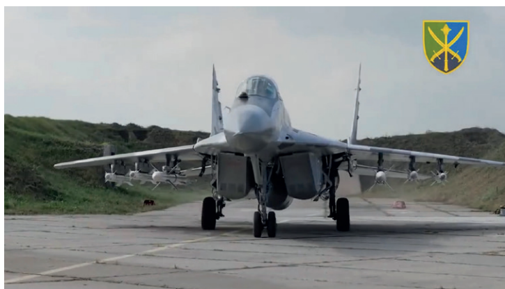
Video shots of the MiG-29MU2 taking off armed with two R-27 and four R-73 rockets.
