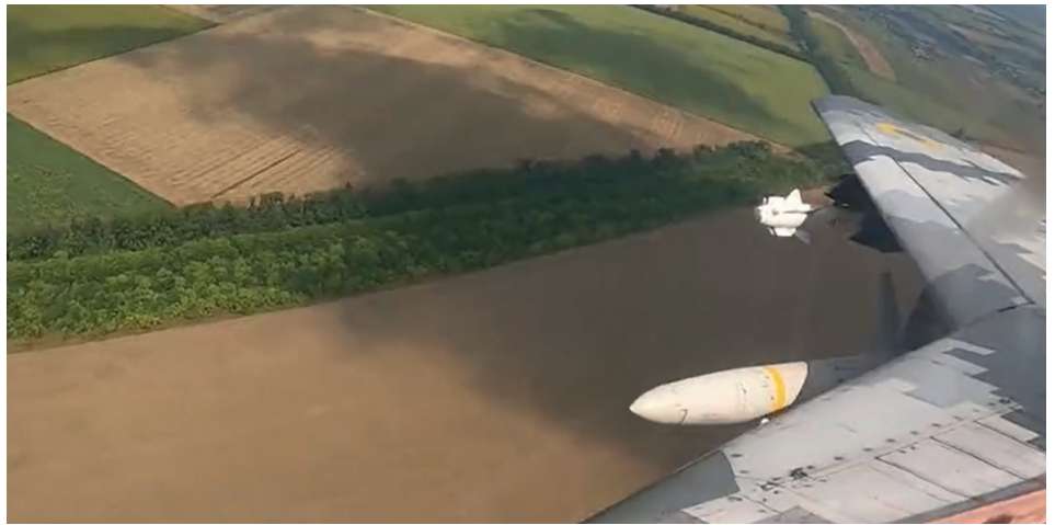
MiG-29 wing showing HARM rocket on the inner attachment and R-73 rocket on the outer attachment. The middle hard point is empty.
