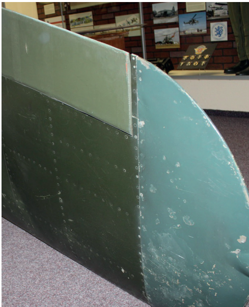
Image of the Skoda-Kauba SK 257 wing fragment from VHU collection: light gray-green paint applied on the aileron fabric covering that may have influenced the Czechoslovak aviation industry after the war. We cannot exclude this paint (of which some stocks could have remained) and its shade as potential application on the Czechoslovak airplanes, including S-199.
