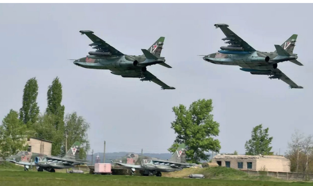
Russian Su-25s usually carry two auxiliary tanks and two B-13L rocket launchers, each with five 122 mm caliber missiles. Ukrainian Su-25s usually carry four B-13L rocket launchers in addition to the tanks.
