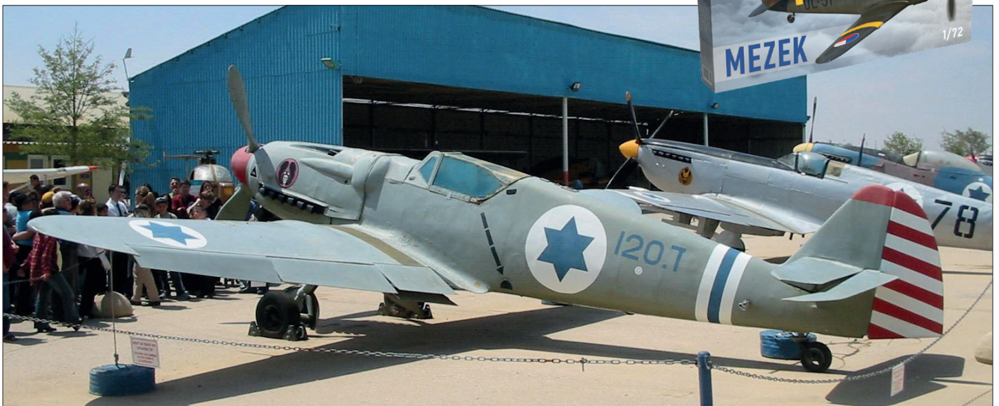
April 7, 2004: With no clear UV coating applied to the newly painted airframe, the D-120 faded to an overall gray color in less than a year...
