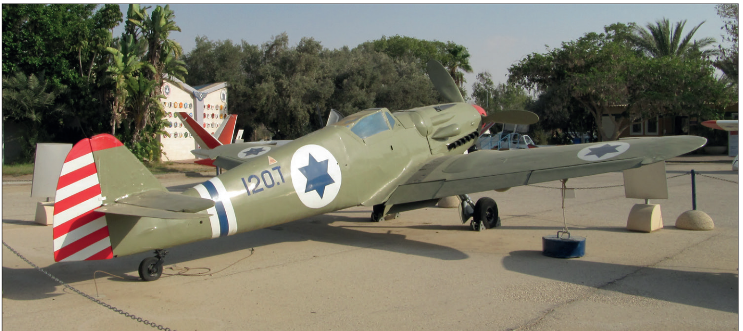
April 7, 2004: With no clear UV coating applied to the newly painted airframe, the D-120 faded to an overall gray color in less than a year...
