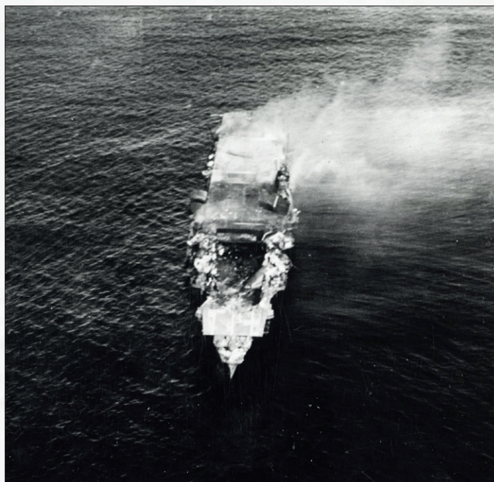
The burning Japanese aircraft carrier Hiryū, photographed after Battle of Midway by a Yokosuka D4Y "Judy" from the carrier Hōshō shortly after sunrise on June 5, 1942. Hiryū sank a few hours later. Flight deck is torn out by the bomb dropped by SBD bomber.
