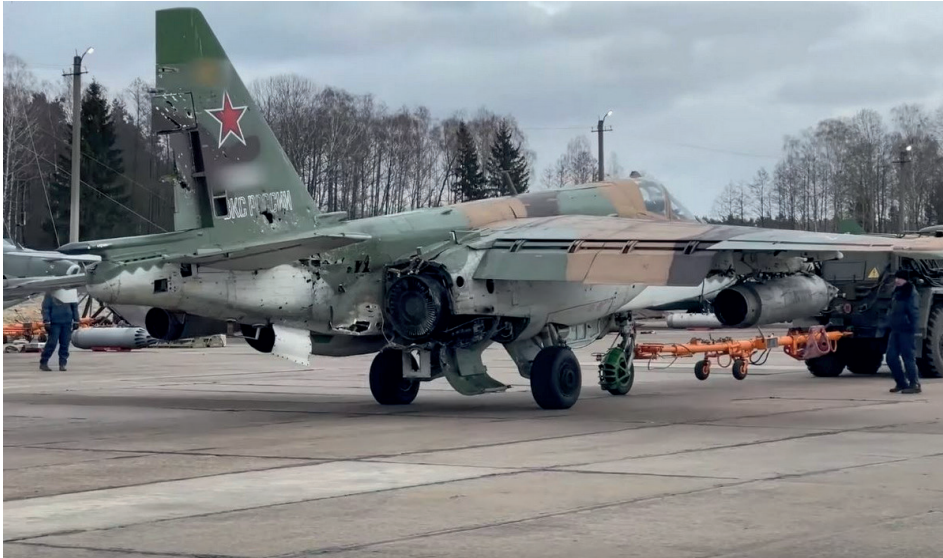
Russian Su-25 that managed to land after being hit by a Stinger in the right engine.
