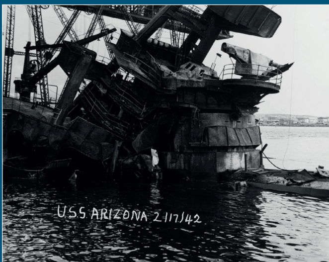
At the first stage of salvage operations the destroyed superstructures were removed. The photograph dated February 17, 1942 shows the superstructure under the forward mast twisted on the gun turret No.2. (photo: Naval History and Heritage Command)
