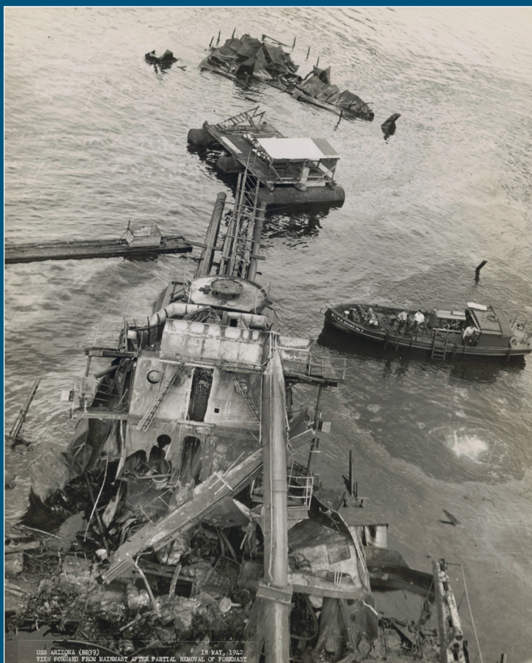
The picture dated May 18, 1942 shows the ship's bow whose center, after the fatal ammunition magazines explosion, collapsed between gun turrets No. 1 and 2 and sank. The forward mast remnants, partially sunken gun turret No. 2 and bow sticking out of the water can be seen (photo: Digital Archives of Hawaii).
