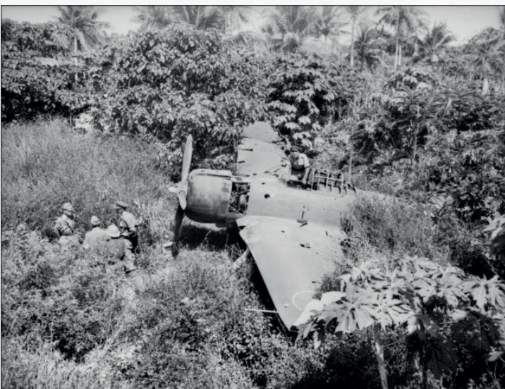
In this October 1945 photo, Japanese and Allied soldiers discuss (at Kavieng airfield?) near the wreck of an A6M2 on the island of New Ireland. Note the green paint applied in field conditions, the white outline of hinomaru on the upper surfaces and the absence of the yellow identification stripe on the leading edge of the wing.
