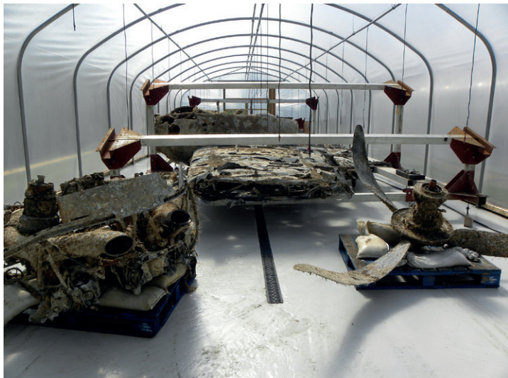
During the period of 2 years the aircraft components have been treated with citric acid indoors the special tents.
