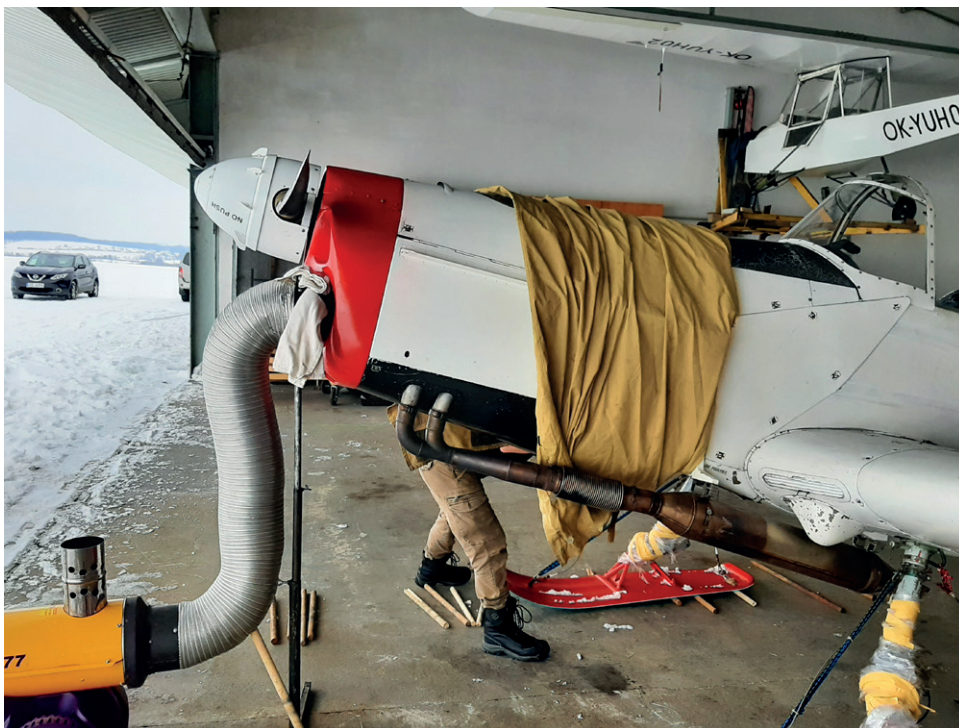
Prior to winter flying, it is necessary to warm up the oil tank in the wing, and then the engine itself.
