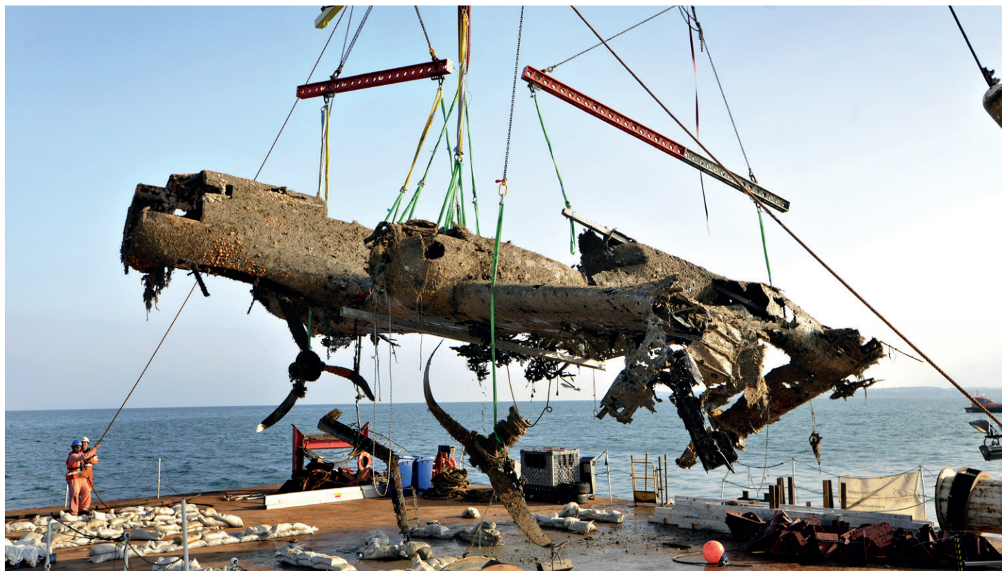
The wreck was carefully laid down on the stand-by barge using the crane.
