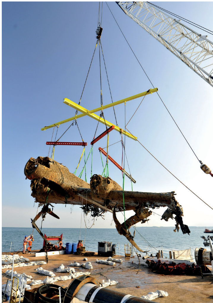
The wreck was carefully laid down on the stand-by barge using the crane.
