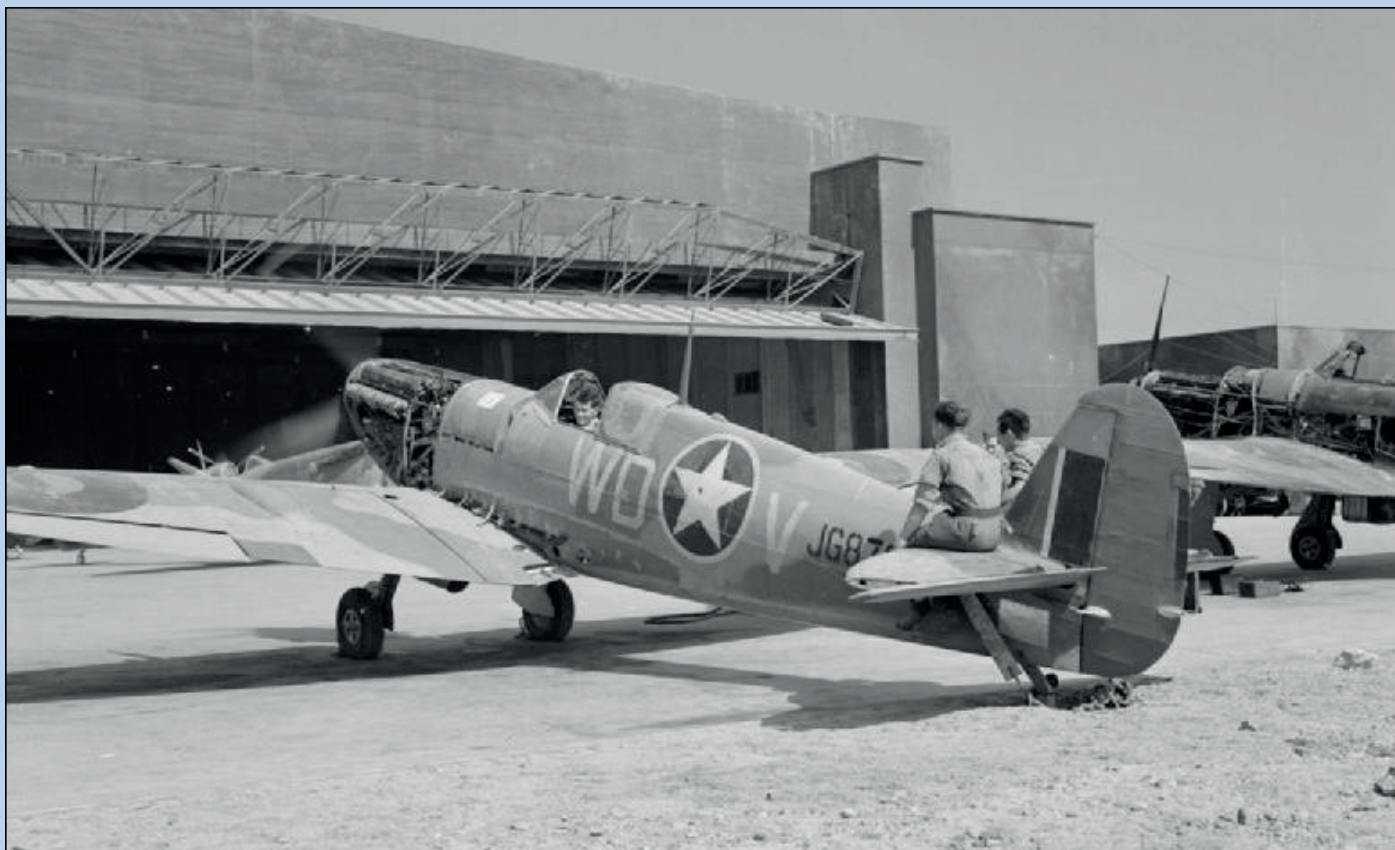
RAF fitters running a test on an overhauled Rolls Royce Merlin engine installed in a Supermarine Spitfire Mk.Vc (possibly JG 873) undergoing repair at No. 144 Maintenance Unit, Maison Blanche, Algeria. The aircraft still sports the markings of the 4th Fighter Squadron/52nd Fighter Group, 12th USAF, with whom it formerly operated (Photo: IWM).
