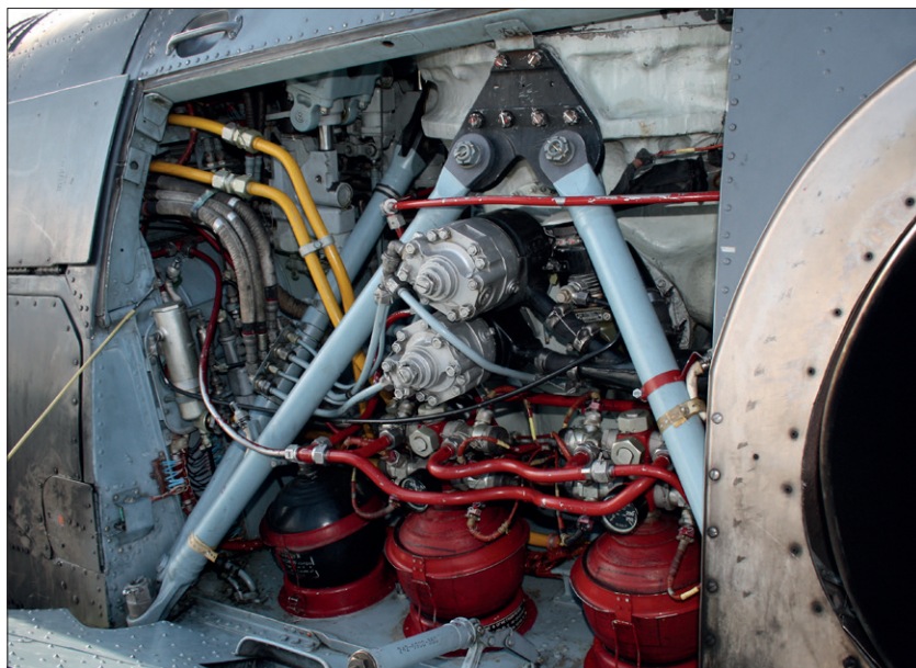
The red cylinders of the fire protection system are located on the right side of the reducer on both the D and V versions.
