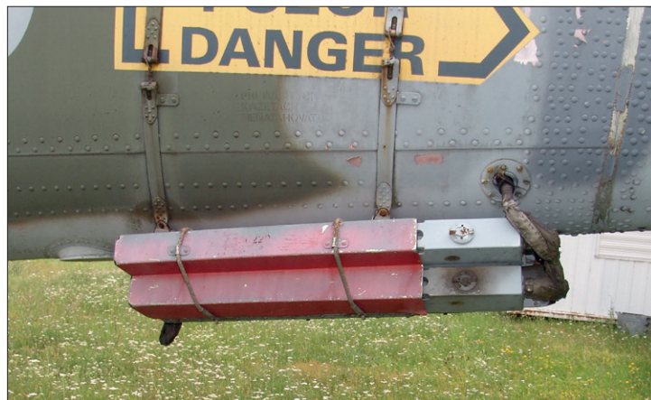
The ASO-2V decoys were retrofitted under the tail spar on the Mi-24D. On the V version, they were already moved to the fuselage because the original design increased the load on the tail spar.
