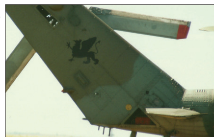
Tailend of the V version with air intake grille for Ai-9V unit. The D version does not have it.
