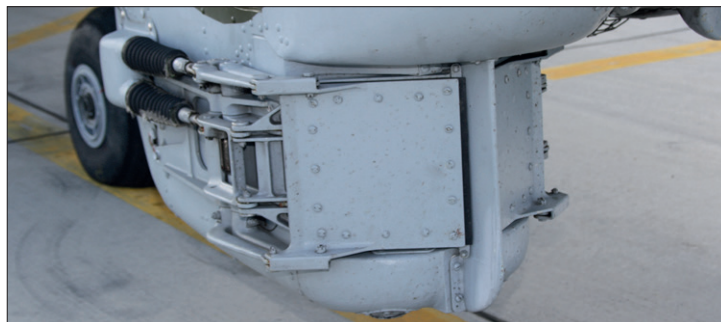
This is what the double cover of the guidance system looks like on the V version.
