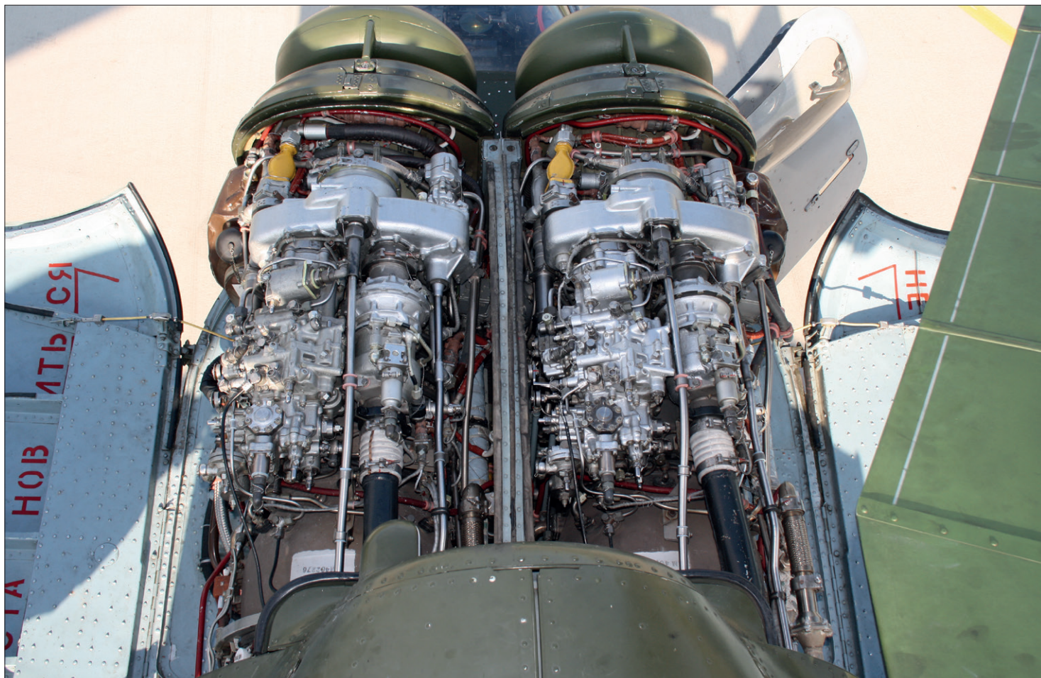
The TV3-117 and TV3-117V engines do not differ from the outside.
