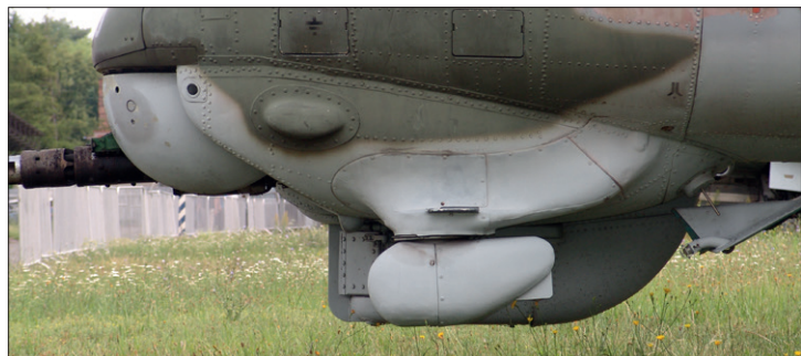
The antenna of the Raduga-F guidance system for the Falanga missiles has a different shape compared to the V version and the whole housing is rotatable.
