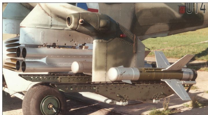
In the picture with the Falanga training missiles, the S-13 gun camera is clearly visible. It was also there on the early Mi-24s delivered to the Czechoslovakia (Nos. 0701 to 0710). In the later choppers it was moved to the cockpit next to the helicopter captain's sight.
