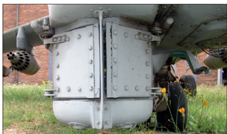
In version D, the optical guidance system housing has only one "door", i.e., the protective cover. In the V version there is also a hinged glass cover underneath. This is closed during observation and preparation for firing and is opened only for the necessary time when the missile is being guided to the target. This ensures that the visor remains as clean as possible and ensures optimum visibility in the viewfinder.
