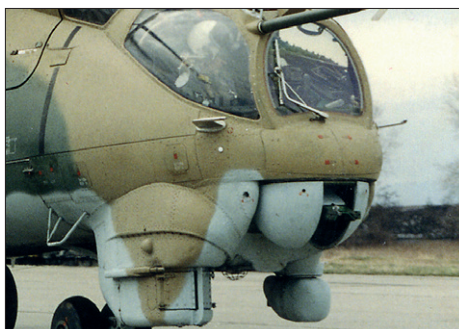
The three-fingered antenna of the IFF SRO-2 Chrom system on the cabin frame at the root of the DUAS sensor tube can be clearly seen in this picture, as well as the retrofitted GPS receiver antenna next to it. The helicopter No. 0214 has the machine gun removed on the picture.
