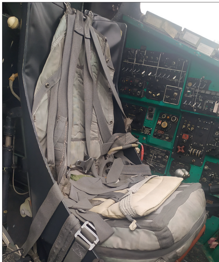
The seat is identical in both versions, the left side of the cockpit differs in the D and V versions more or less only by the radio control panel.
