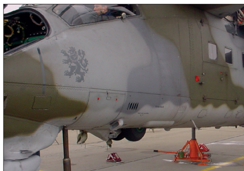
The Hind D on the support stands during hydraulic system testing. In the picture you can clearly see the absence of the landing light on the lower left part of the fuselage under the captain's cabin.
