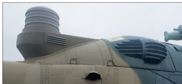
Unlike the V version, where the air intake for the Ai-9V auxiliary power unit is routed through the tail via the grille at the SARPP-12DM emergency recorder, the D version has the intake directly at the power unit on the right side of the fuselage. Also shown is the retrofitted L-166V-11E.
