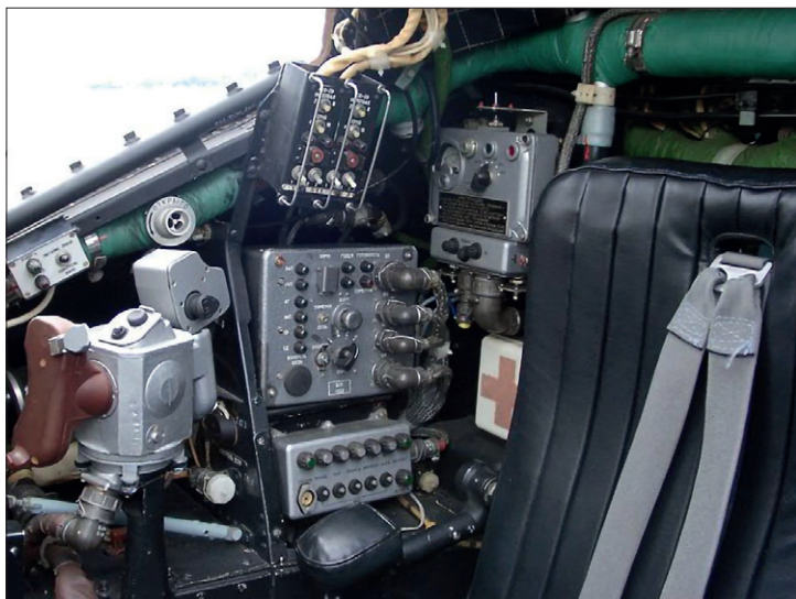
The bigger differences are on the right side, where the control consoles and controls for the Falanga anti-tank missile system are located. The L-166V-11E infrared jammer control box is located above the "rams".
