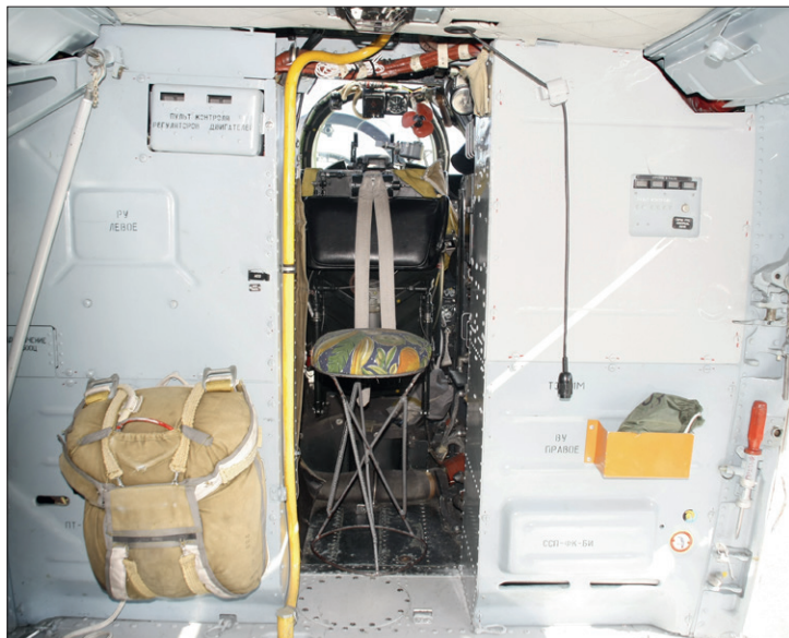
A view of the version V tunnel. Note the elegant tripod for flight engineer. The parachute hanging on the left side is also for him.
