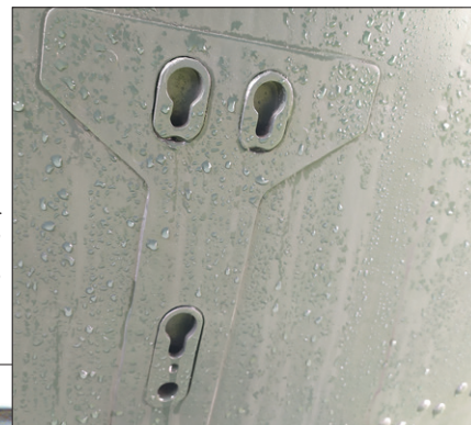
T-shaped bracket for mounting the winch for hanging armament. The V version does not have it.
