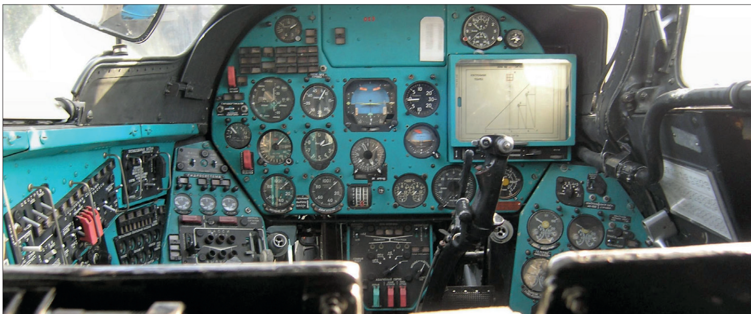
View of the Mi-24D instrument panel, with the center section covered by plate and with uninterrupted top cover. The gunsight is mounted on the cockpit frame. The lower armament panel can also be clearly seen, which differs substantially from the V version in the arrangement of the controls.
