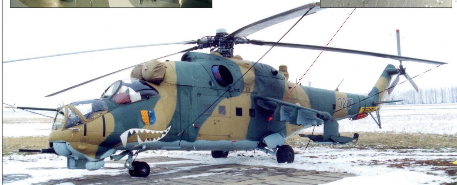
The lack of trim around the exhausts is clearly visible in the picture. These are only on the V version. Also missing are the mounting points for the EVU device above and below the exhausts. Also different is the shape of the exhausts themselves, which did not have to be cut for D version to install the EVU exhaust gas cooling system.
