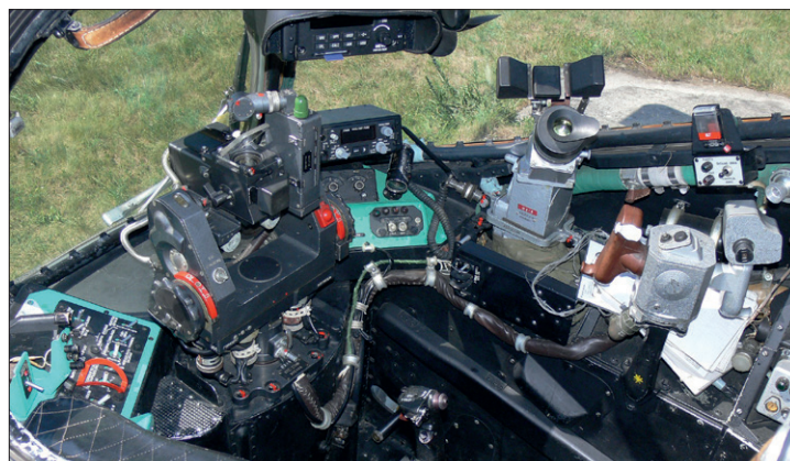
The front panel in the pilot-operator cabin is dominated by the KPS-53AV aiming station. The panel to the left of it is identical to the V version, the right one is slightly different. The photo of the cabin of 0215 chopper shows the retrofitted equipment - GPS unit on top and radio below.
