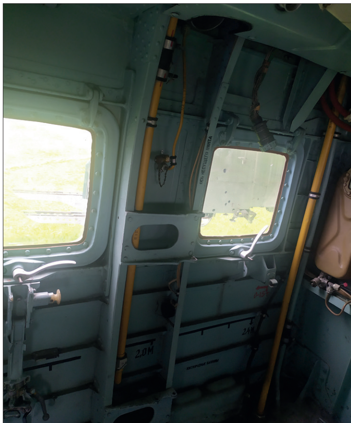
Below the two air conditioning outlets, the opening for the filling of the internal auxiliary tank can be seen.
