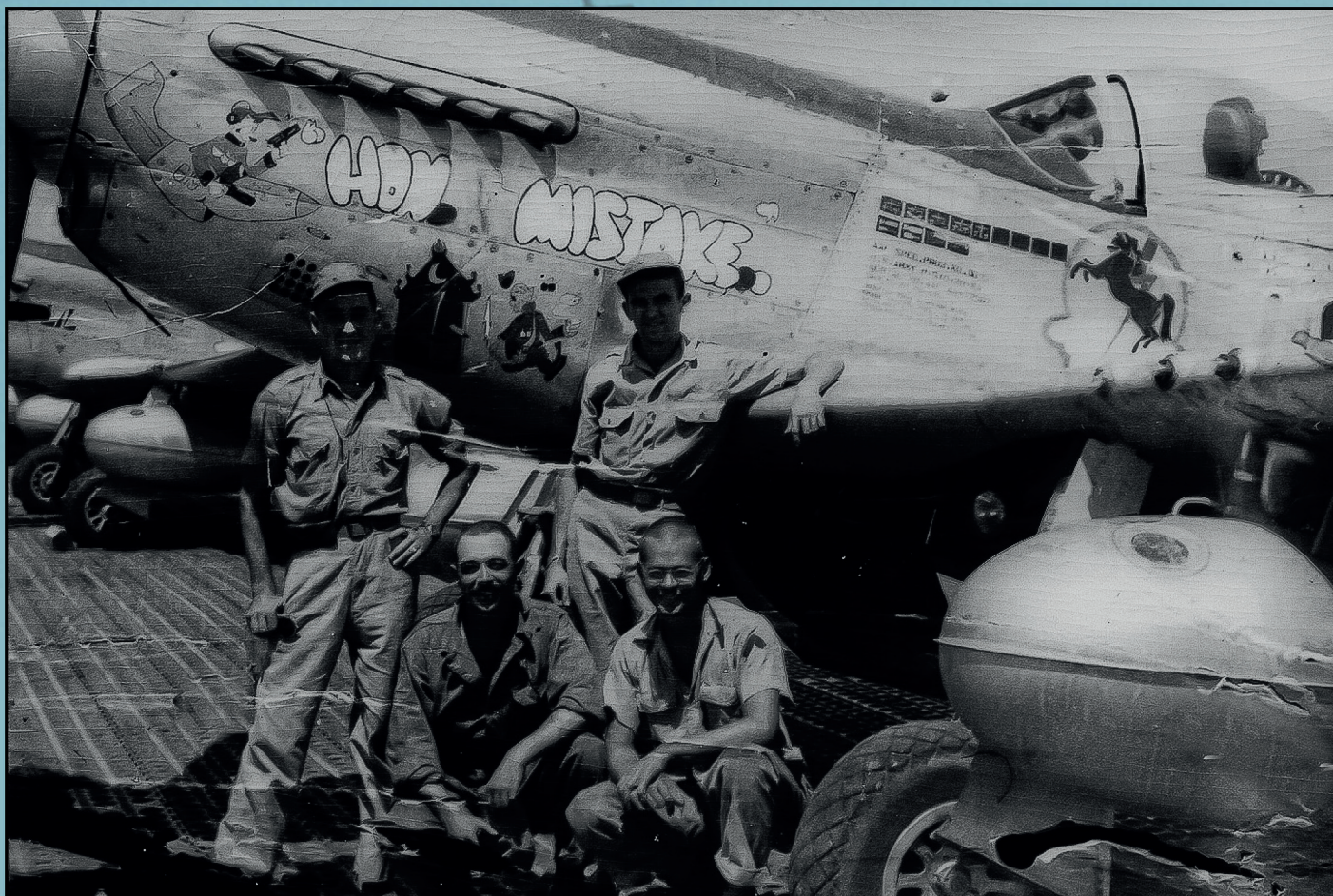
Bill Ebersole and Jim Bercaw, along with two of the ground crew members for 'Hon. Mistake'. Here the airplane has the 110 gallon drop tanks attached, and you can see the mission symbols for the long range missions to Japan as well as the ground attack sorties to Chichi Jima.
