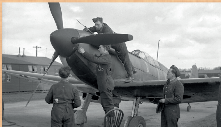
No 602 Squadron Spitfire Mk.Ia flown by P/O A.A.McKellar during maintenance. See the anti-spin fairings on the sides of the fuel tank cowlings.
