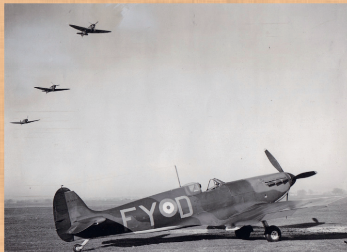
No 611 Squadron Spitfire Mk.I equipped with armored windshield.
