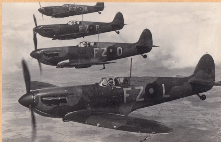
No 65 Squadron Spitfire Mk.Is. The aircraft are equipped with two blade propellers, bulged canopies without the armored windshield, early type of the Pitot tube and the early antenna mast.
