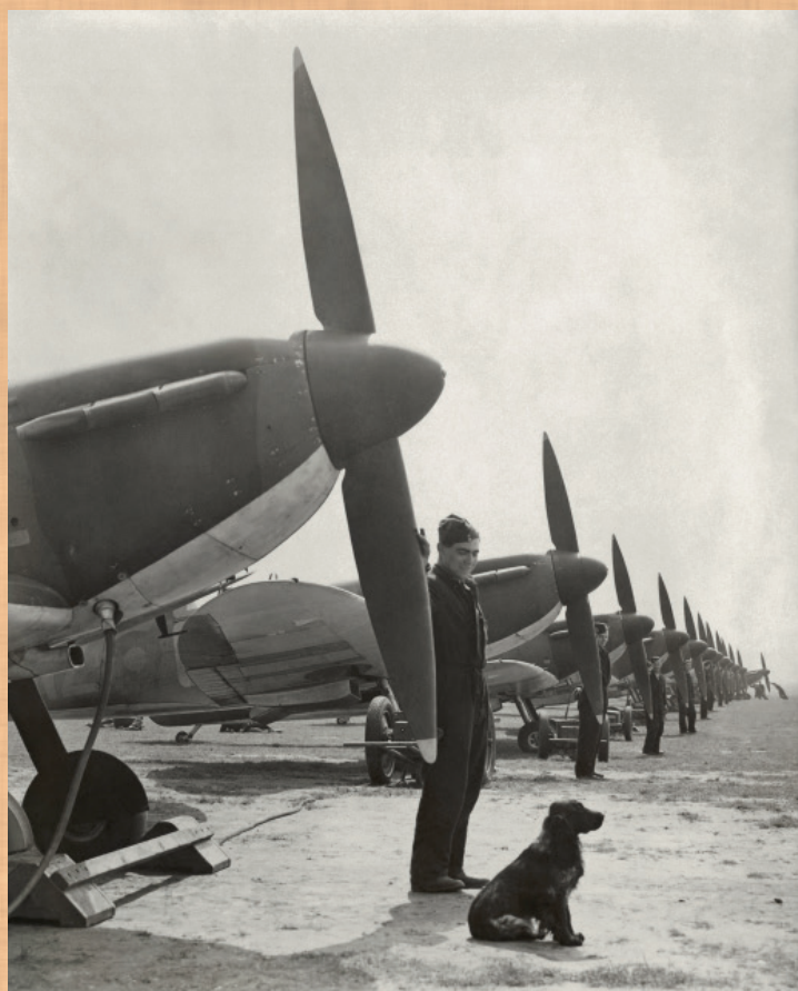
No 19 Squadron Spitfires equipped with late type of the Pitot tube, and already by the hot-air gun heating.
