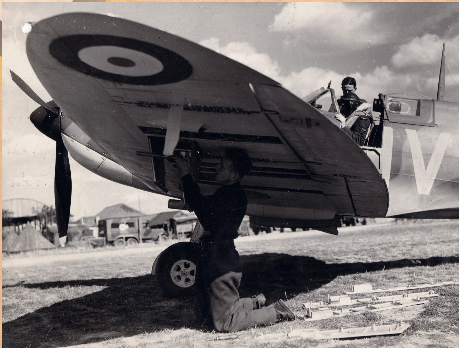
Spitfire Mk.Ia of the No 19 Squadron with full armor, gun heating, late type of the Pitot tube and three blade De Havilland Type 5/20 propeller.
