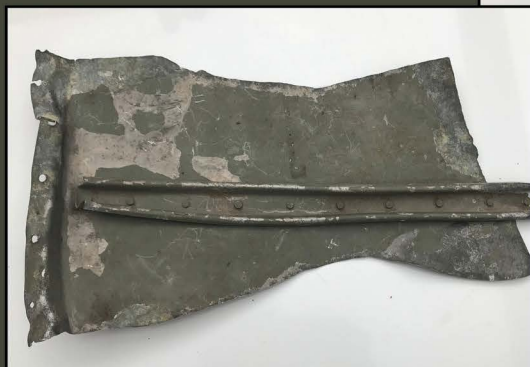
Part of the tail surfaces of the machine of Koepsell and Schmidt. On the inside, a protective coating in the shade RLM 02 is visible. On the outside, a red color is painted for unknown reason over the pale blue RLM 65. Photo: Stephen Newman
