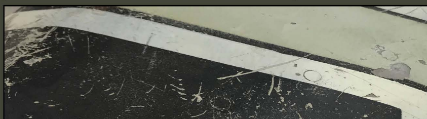
Part of the tail surfaces of the machine of Koepsell and Schmidt. On the inside, a protective coating in the shade RLM 02 is visible. On the outside, a red color is painted for unknown reason over the pale blue RLM 65. Photo: Stephen Newman
