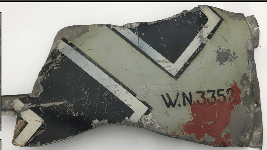
Part of the tail surfaces of the machine of Koepsell and Schmidt. On the inside, a protective coating in the shade RLM 02 is visible. On the outside, a red color is painted for unknown reason over the pale blue RLM 65. Photo: Stephen Newman
