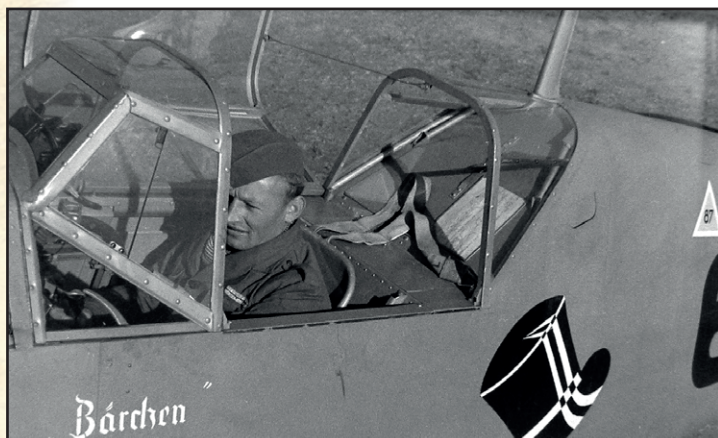
Source: Hanns-Wolrad Dölling via Erik Mombeeck coll. In this picture, we can appreciate the details of the 'Bärchen' inscription, and note the lack of the pilot's head armour, which was not installed in the Messerschmitt Bf 109 E during this period.
