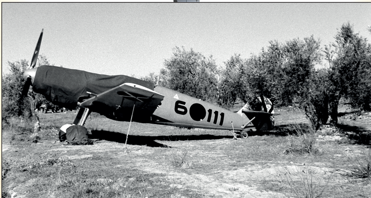
Source: Hanns-Wolrad Dölling via Erik Mombeeck coll. Bf 109 E-3 coded 6•111, seen at La Cenia airfield during its initial period of service. The engine and cockpit area, as well as the main wheels, are covered with tarpaulins to protect from the sun.
