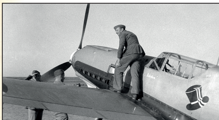
Source: Erik Mombeeck coll. Another photo of 6•111 with ground crew reveals the dark finish of the supercharger air intake, which was usually left in RLM 71 as supplied from the factory. Also note the dirt collected in the wing root area, and chipped black paint on the foothold.
