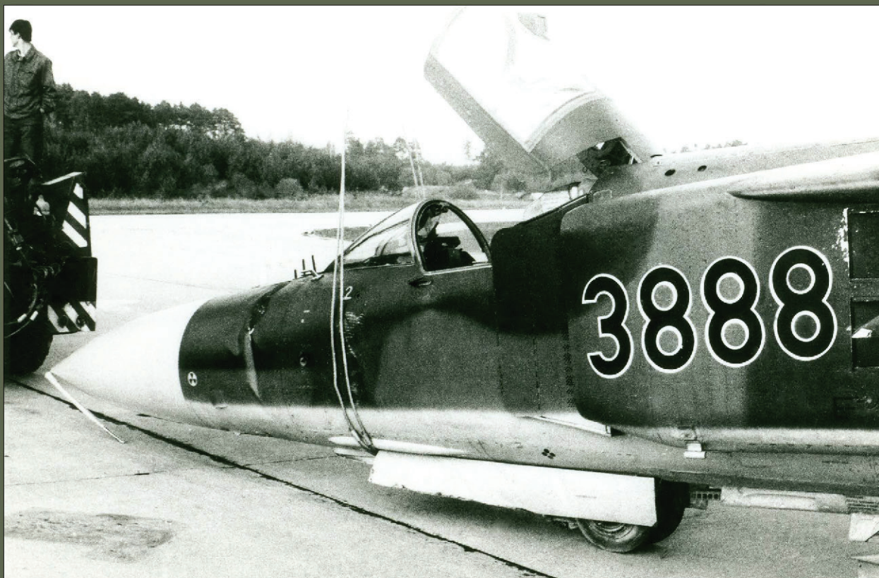
During the landing, the aircraft suffered a collapsed nose gear, destroyed infrared sensor and damaged radome. Most importantly, though, the fuselage suffered warpage.
