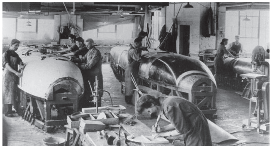
The Mosquito's fuselage was produced by forming timber strip laminates over a concrete buck. When cured, the halves were fitted out and glued together, much like a plastic model kit.
