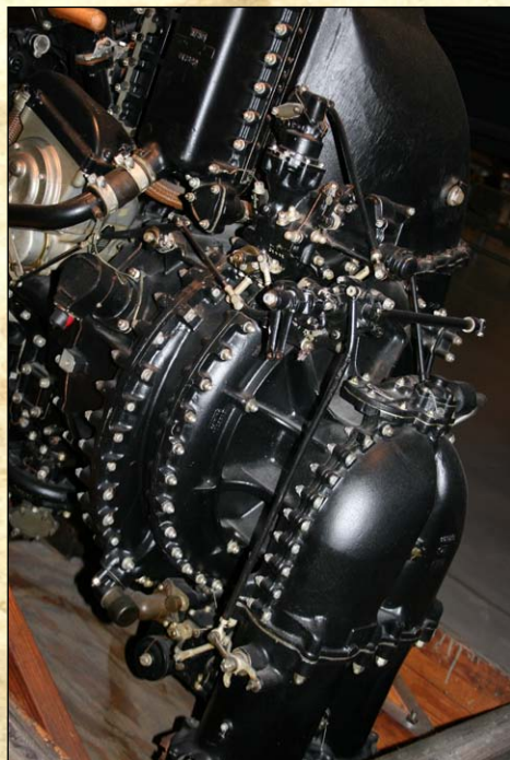
One of the components that greatly favored the RR Merlin over the competing engines, is the two-stage supercharger located at the rear of the unit.
