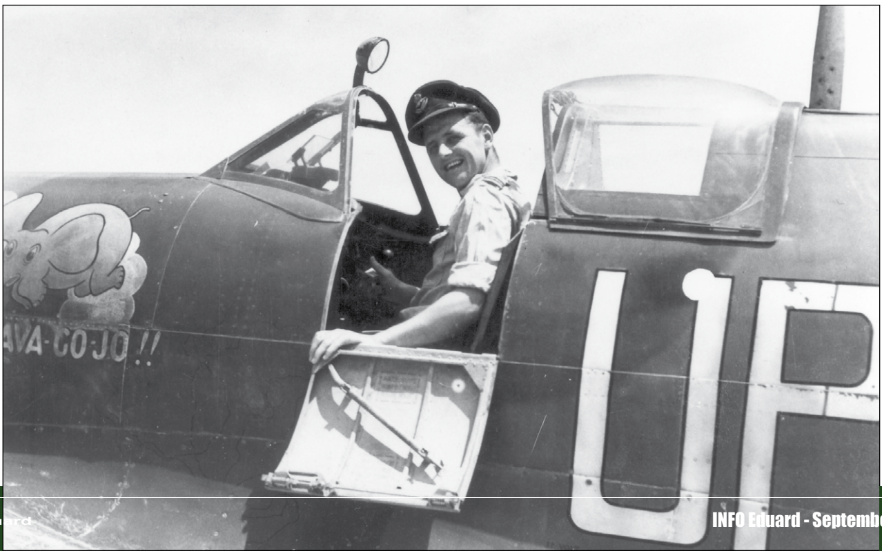
Norm cracks a broad grin for the cameraman. Noticeable in this photo are the black pin striping around the code letters, the fading and chipping of the code letters, and the 'shadow' left by the 'arms' of the stencil when painting the 'P'.
