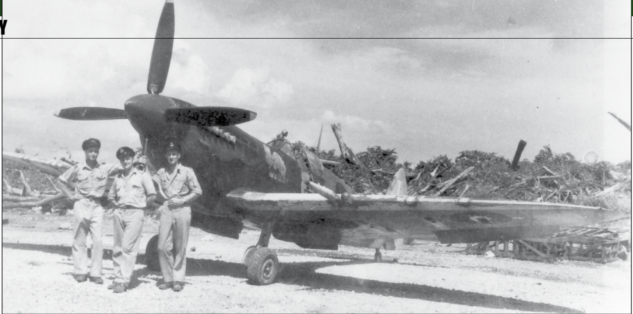
Norm with Flying Officer Doug Edwards, at left, and Flight Lieutenant Len Reid DFC, at right, pose in front of A58-517 in June 1945. The ravages of three months operational service are now readily apparent. As well as having been eroded from the empennage, the White paint on the wing leading edges has also become badly chipped and worn, allowing sections of the original RAF Yellow leading edge paint to show through on the outer part of the wing.
