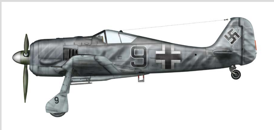
Focke-Wulf Fw 190 A-3 „black 9“ of 2./JG 5 at Stavanger-Sola airbase, July 1942. The digit painted on undercarriage cover is typical for 190s of I. and III./JG 5. This fighter plane got a „tiger“ camouflage and ETC 501 rack. Both features are unusual for this unit and period of war. (Profile: Kjetil   kra)
