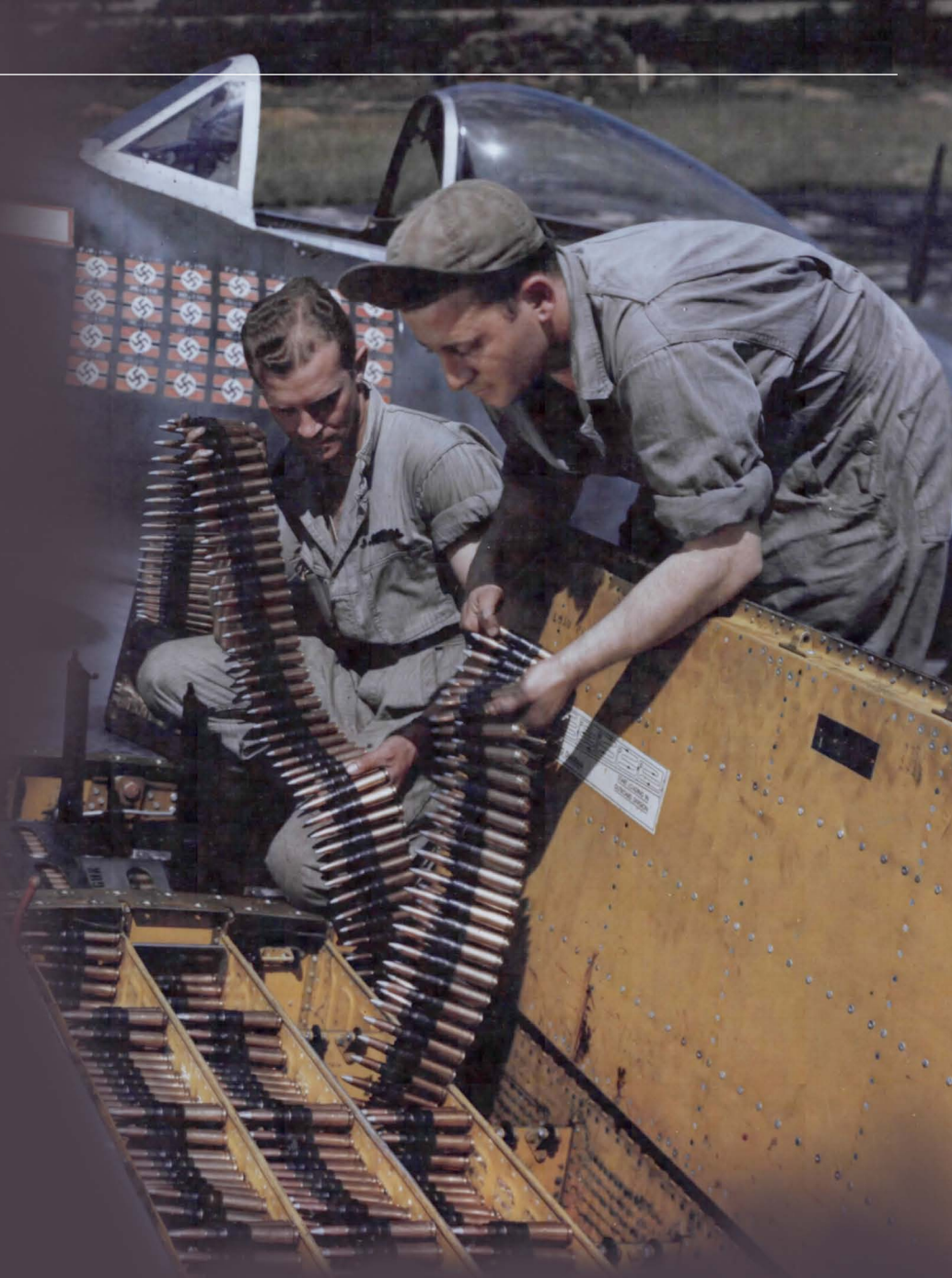
▲ Installation of ammo belts for the 0.5in AN/M2 in the P-47 and P-51.
