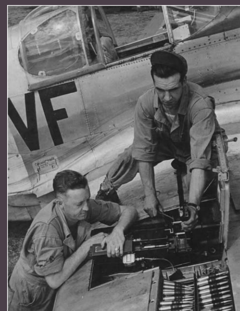
▲ Installation of ammo belts for the 0.5in AN/M2 in the P-47 and P-51.
