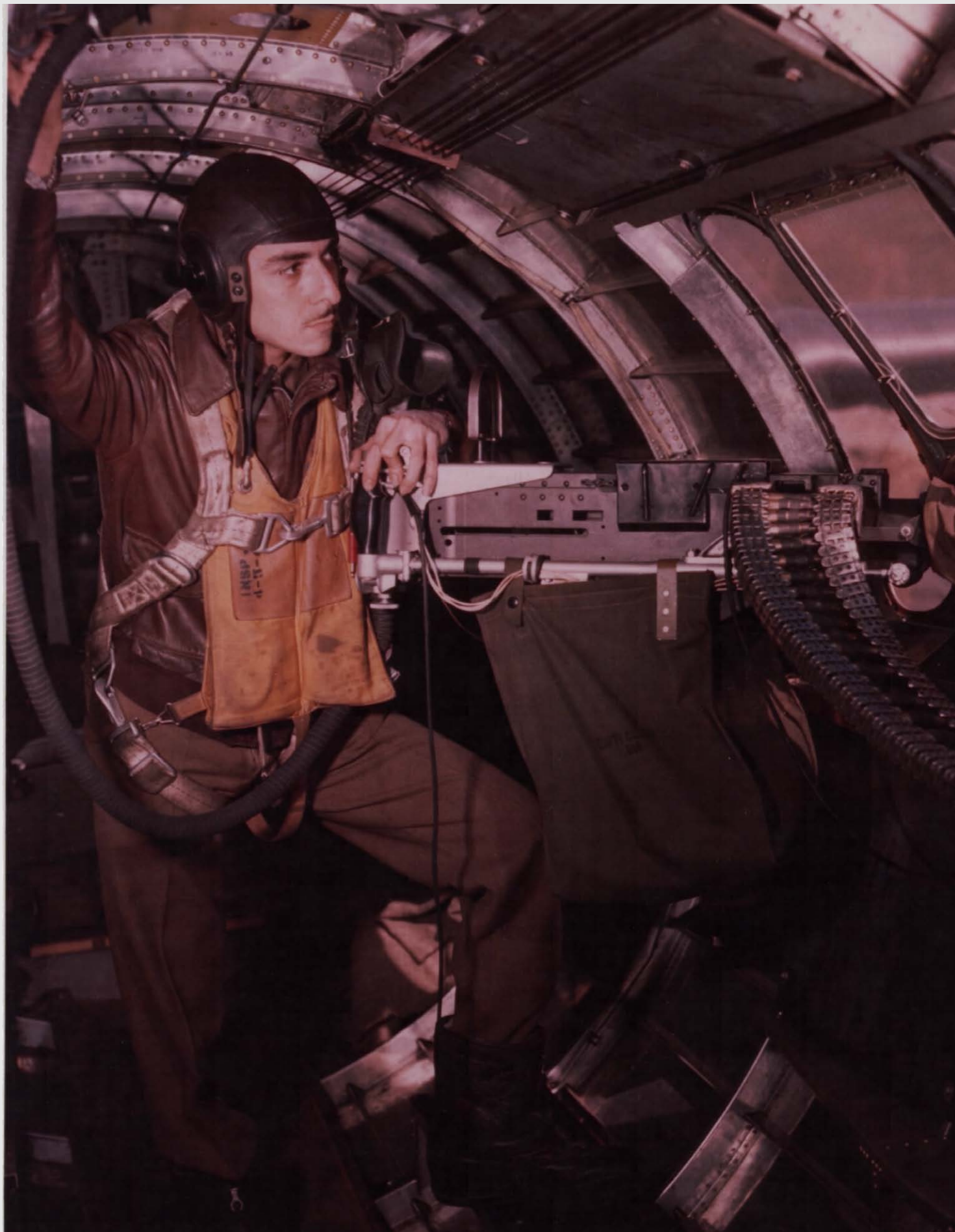
Waist gunner on his position in the B-17G series mid production with the divided, but already closed waist window (NARA)
