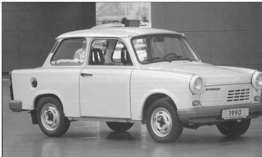
✦ The last version to be produced, the Trabant 1.1 with a four cylinder, four stroke engine from VW. The rad cover reminds of another East German vehicle, the Wartburg.
