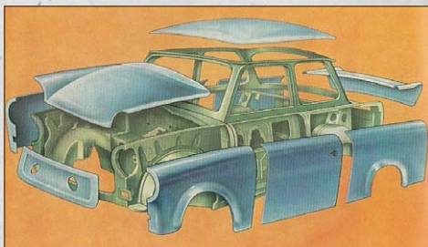
Plastic components mounted on a steel skeleton.
