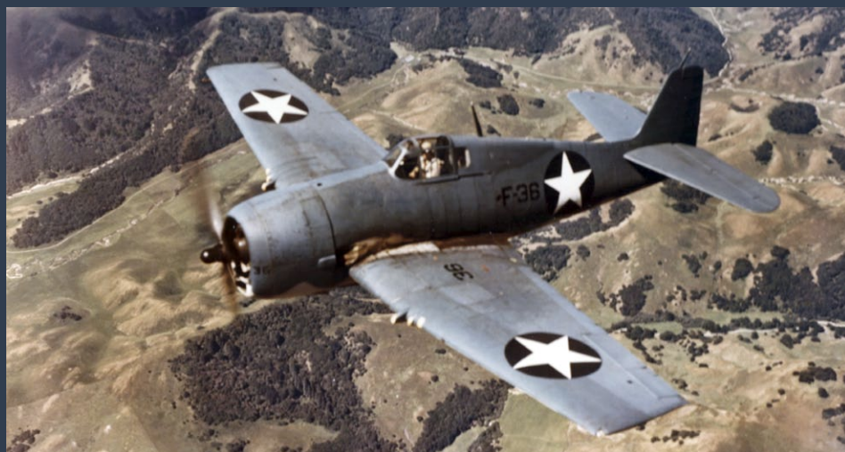
An F6F-3 in flight during 1942. Early Hellcats had Non-Specular Blue Grey camouflage on the upper surfaces with simple stars (no bars). Note that the paint is heavily faded.
