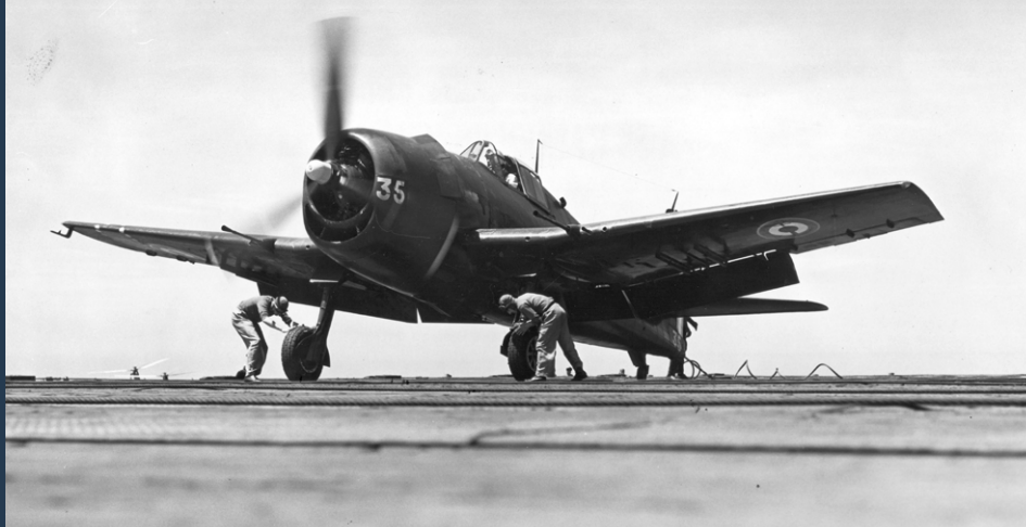
An F6F-5N in French service. These post-war French machines may easily be identified by their additional cannons.
