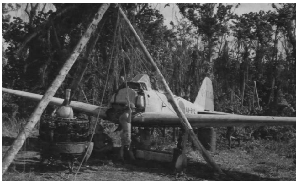
American intelligence had a field day at Buna. There were at least thirteen Reisen on the ramp in various states of disrepair. Two of them were passed on to a second opinion in Australia. Aircraft „Q-102“ was inspected right on the premises at Buna. The photo shows the Sakai 21 engine that has clearly seen better days, and the oil tank is visible on the fuselage bulkhead.
