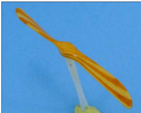
10. Second layer - darker wood grains - on the propeller, applied to the varnished first layer.
