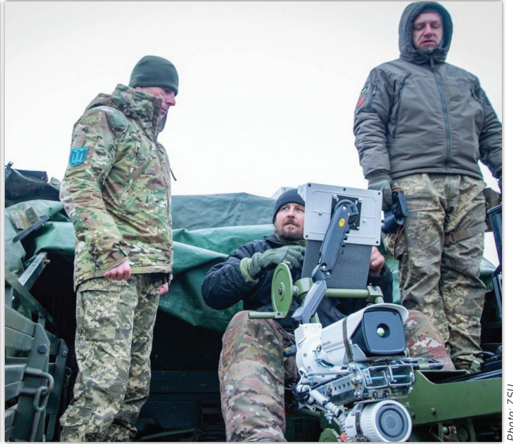
20 mm caliber cannon Zastava of Yugoslav origin which the Ukrainians upgraded by night vision gunsight.
