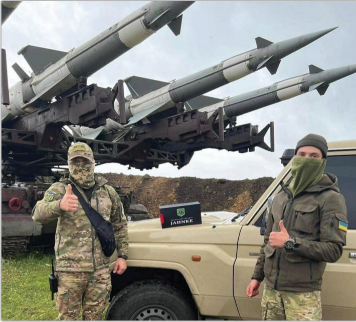
Polish system Neva SC mounted on the WZT-1 tank chassis
