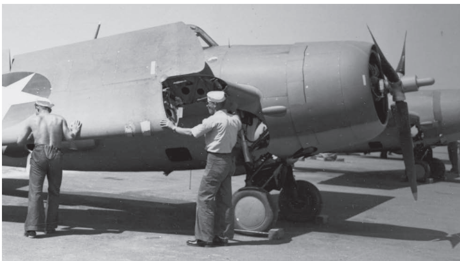
A major innovation in the F4F-4 version was the "So-Wing" folding system, designed by Leroy Grumman himself. Here, mechanics demonstrate the system's space-saving capabilities on an aircraft belonging to VF-3 at NAS Kaneohe, Oahu, May 29, 1942.
