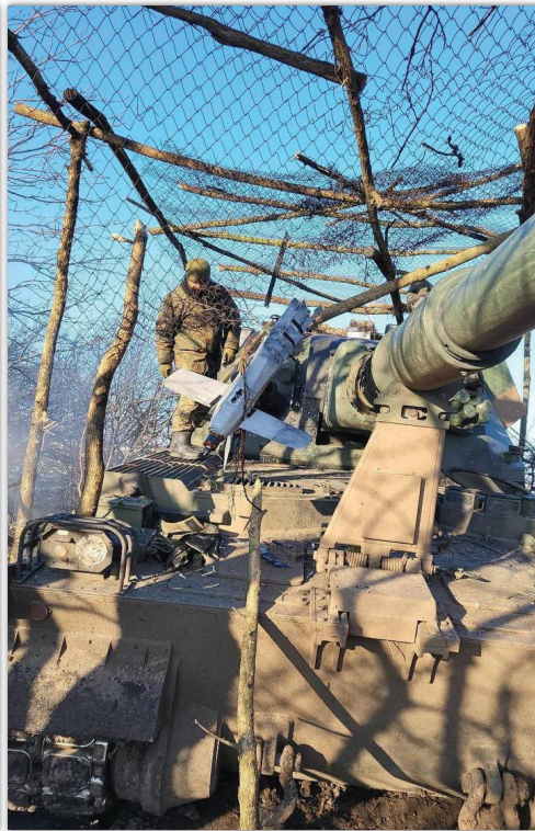
A Polish-made Krab self-propelled howitzer was saved from a Russian Lancet kamikaze drone by a metal mesh.
