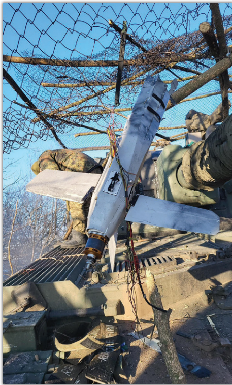
A Polish-made Krab self-propelled howitzer was saved from a Russian Lancet kamikaze drone by a metal mesh.
