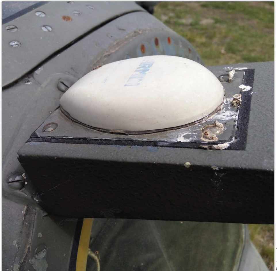
Detail of the GPS antenna fitting developed in LOK.
