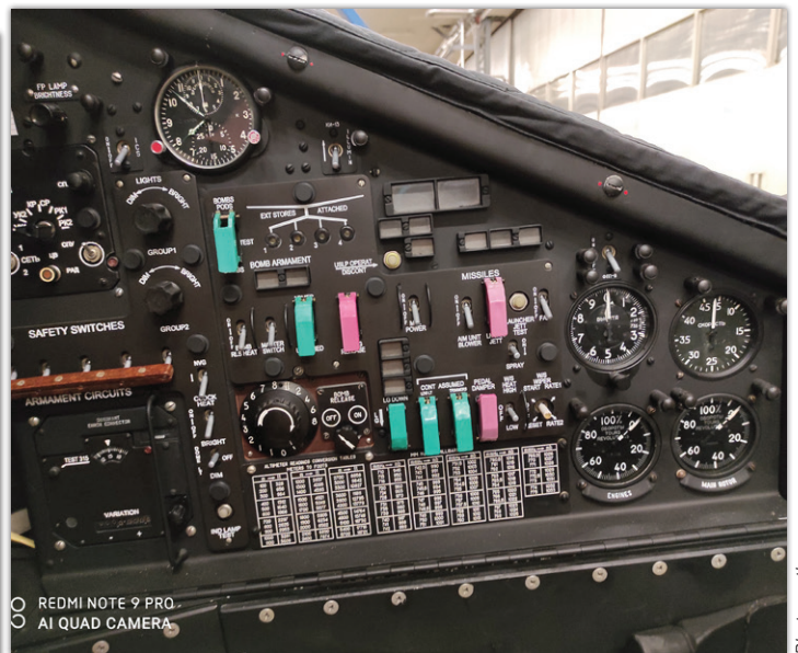
Left side of the WSO's cockpit already in black color with English stenciling and the conversion table from feet to meters. Necessary, as the altimeters were calibrated in meters.
