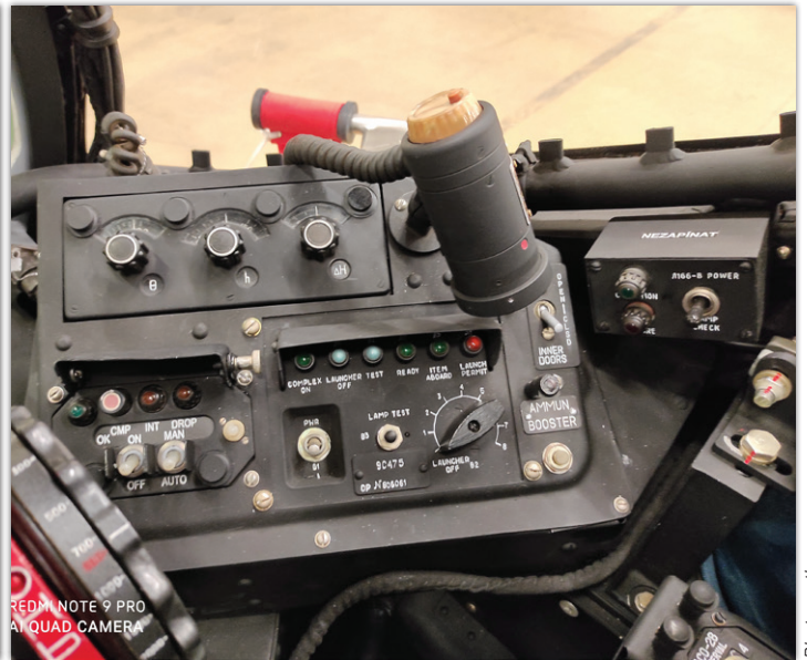
Control panel of the infrared-guided missile countermeasure system L-166V-11E „Isanka“ was located next to the right front weaponry panel in the WSO's cockpit.
