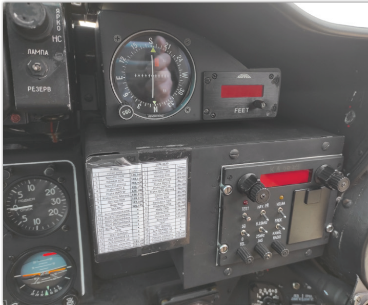
The control panel of the new radio LUN 3520 allowing continuous change of the frequency replaced the Doppler navigation system DISS and the navigational data were instead supplied by the GPS system.
