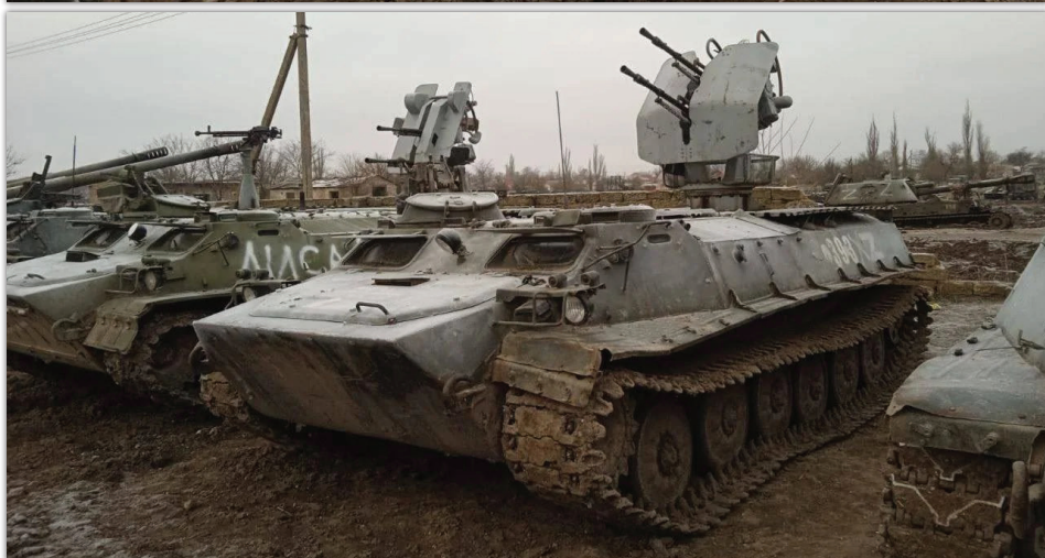
Russian MT-LB with 2M-7 naval turrets with two 14.5 mm caliber machine guns.
