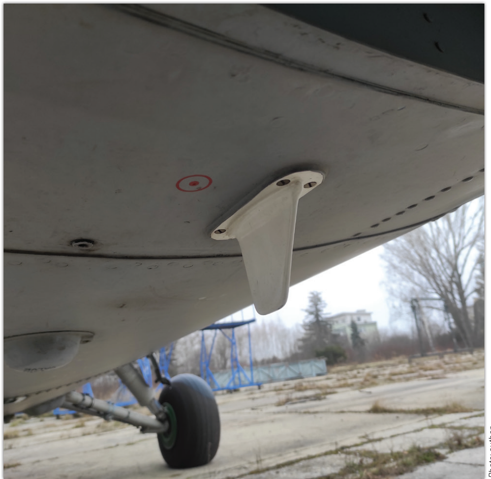
Antennae of the APX-100 transponder were fitted behind the front wheel bay and on the top of the tail boom.
