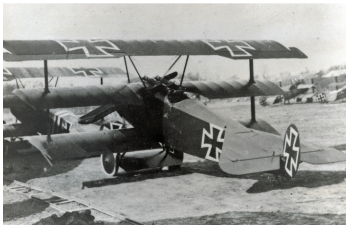
The iconic Fokker Dr. I 425/17 in its initial stage of decoration, marked with Iron Cross national insignia. The smooth opaque application of the red paint indicate that it was most likely spray-painted in this color at the Fokker factory.
