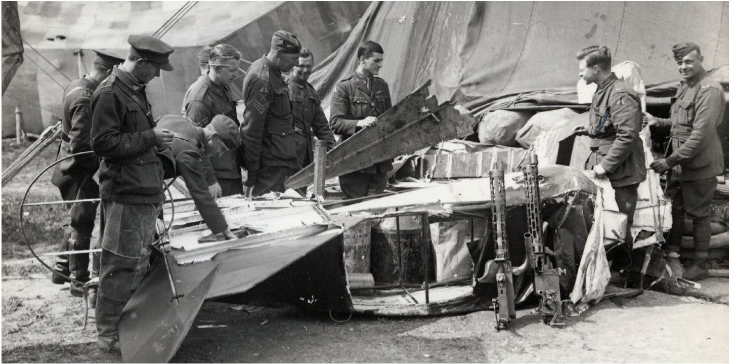
The souvenir hunters had thoroughly taken apart Dr.I 425/17 when this picture was taken. The inner surface of the remaining fuselage fabric show no sign of streaking, supporting the theory that at least the upper and side surfaces of this plane were just painted red at the factory.
