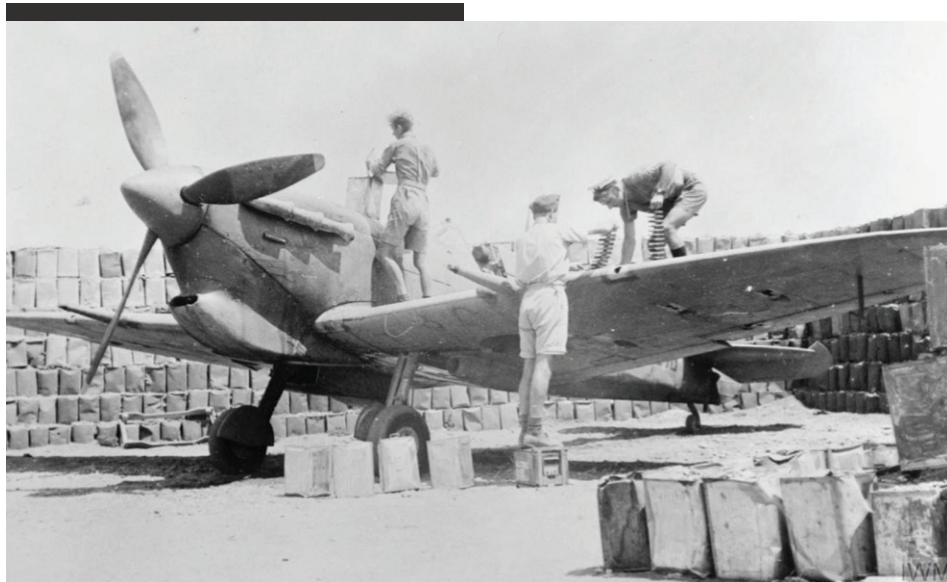
An RAF ground crew refuels and rearms a Spitfire Mark Vc from No. 603 Squadron RAF at Ta Kali airfield. The protective wall was raised from empty fuel cans and sandbags.
