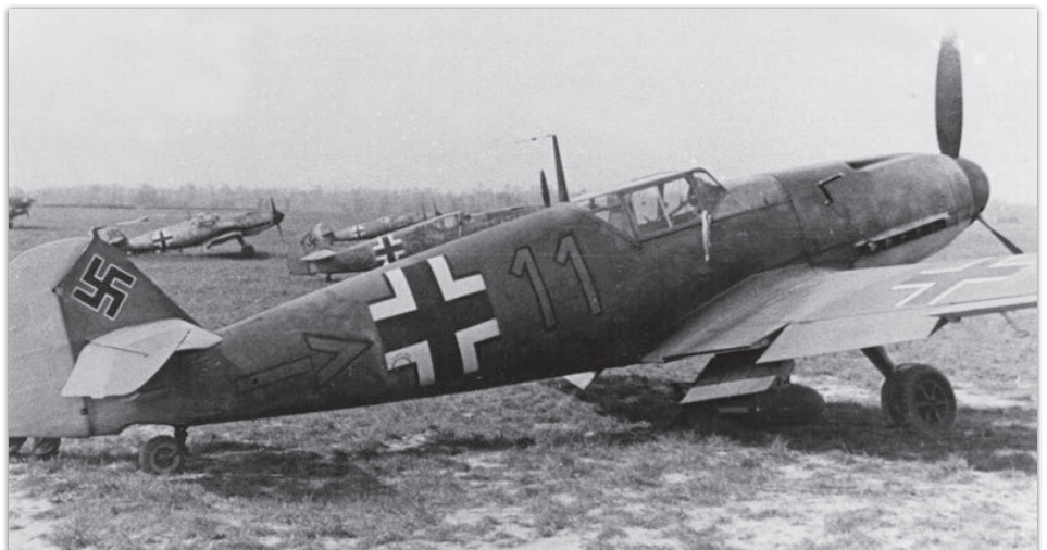
Bf 109 F-4 od 10. (Jabo)/JG 2 in France during the summer of 1942. The aircraft sports reinforcing stringers on the rear fuselage. The photo shows the typical position of the open landing flaps and the combined glycol cooler and landing flaps.
