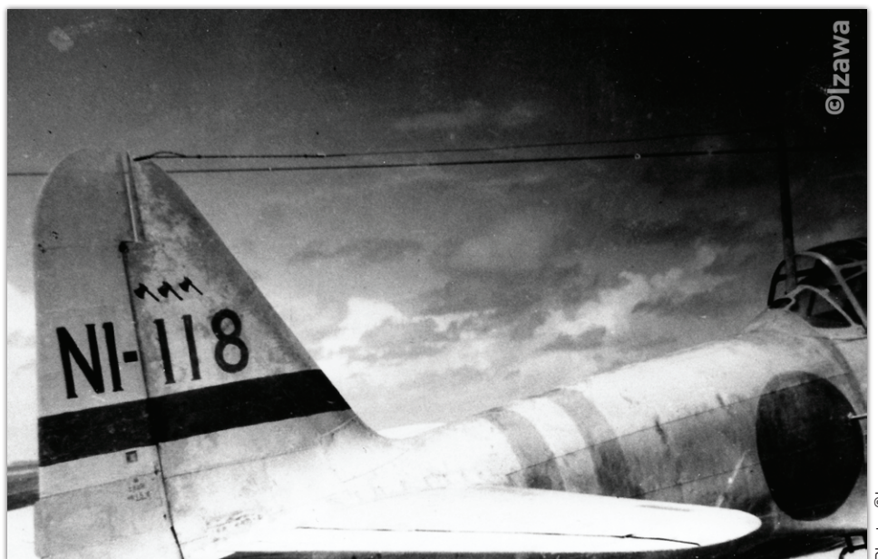
The NI-118 was the fifth Rufe seaplane produced, so it was a rebuilt machine from the A6M2 Model 21 carrier fighter produced by Mitsubishi during its overhaul and rebuild by Nakajima. Pictured here in early 1943, after a year of service, this vintage aircraft shows considerable signs of paint wear. It is possible that the darker areas on the stabilizer are made up of reddish-brown primer.
