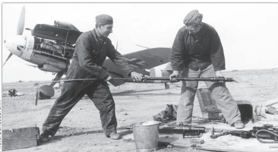
JG 27 Bf 109 F-4 Trop in North Africa. Mechanics are cleaning the barrel of the MG 151/20 cannon.
