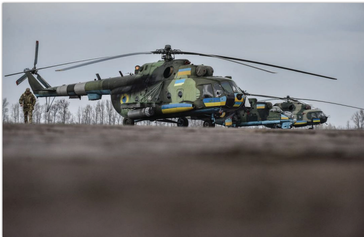
A pair of Ukrainian Mi-8s armed with a machine gun in the nose. Between them is an Mi-24.
