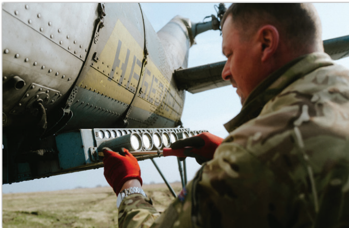
Nice detail of the decoy targets on a Ukrainian Mi-24 helicopter.
