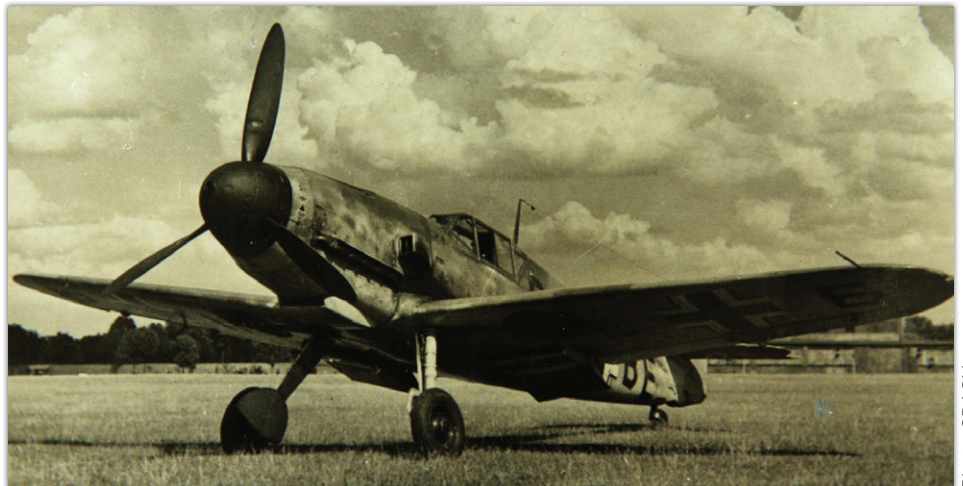
Bf 109 F-0 PH+BE already had oval wingtips, but the intake turbocharger had a rectangular cross-section, characteristic of the Bf 109 F-1 produced by the WNF factory.
