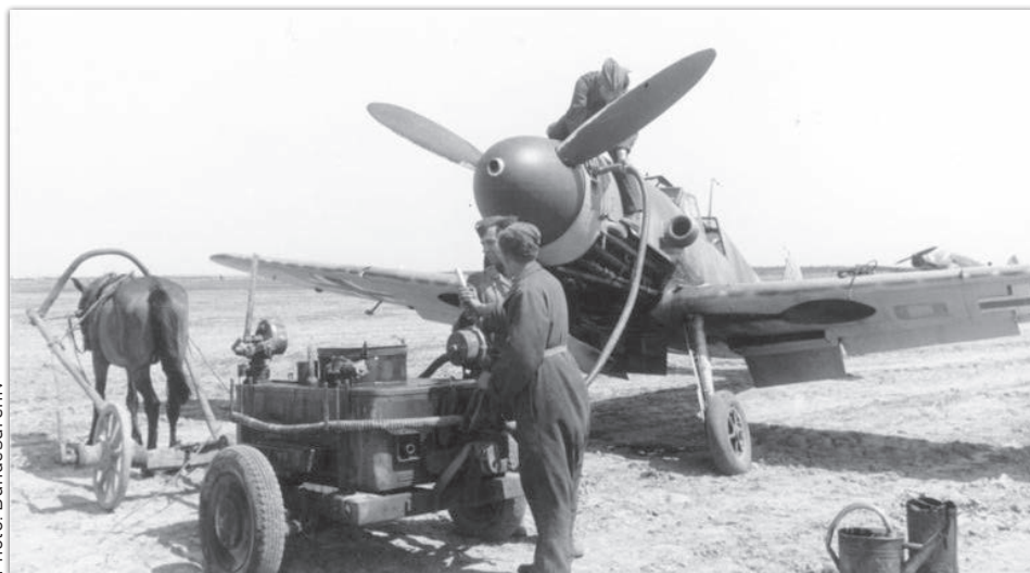
Bf 109 F-4/Z during an oil refill. The aircraft has circular wheel wells, a larger compressor intake and a VDM 9-12087A propeller with wider propeller blades.
