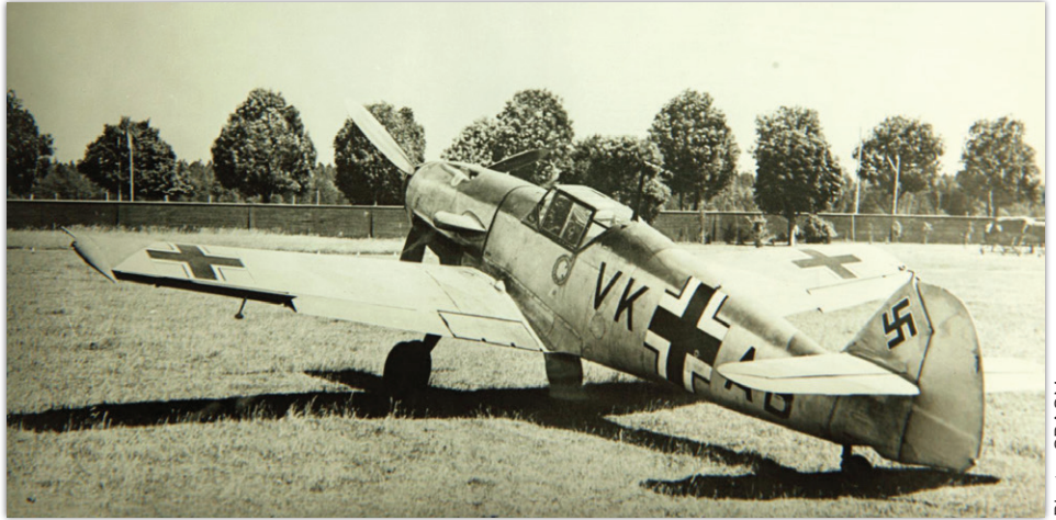
Bf 109 F-0 WNr. 5604 VK+AB. The aircraft with the DB 601 A engine already had the compressor intake with a circular cross-section. It was used to test the newly designed glycol cooler flaps combined with landing flaps. The wing still had the straight ends of the Bf 109E.
