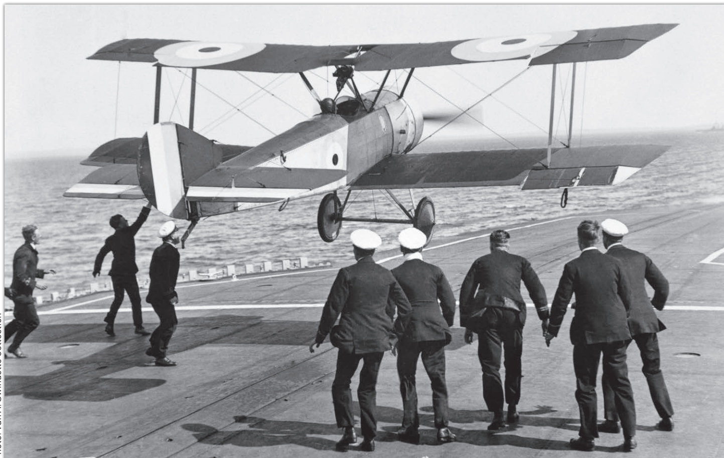
Squadron Commander Edwing H. Dunning flying Sopwith Pup is performing the first successful landing on the HMS Furious deck on August 2, 1917, during the trials in Scapa Flow. The ship was sailing at 26 knots with 21 knots headwind. That provided 87 kph headwind speed on the deck therefore the airplane flew at very low speed relative to the deck. Five days later, during the third attempt to land, Dunning crashed into the sea and perished.
