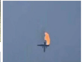
Burning IL-22M shortly before crashing into the ground. The tail, the outer wing parts, and both outer engines were torn off during the fall.
