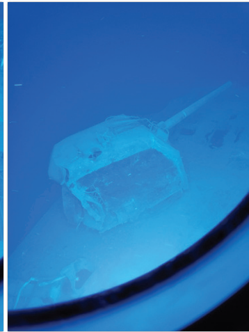
The rear gun turret of USS Samuel B. Roberts featuring the 127 mm caliber cannon.
