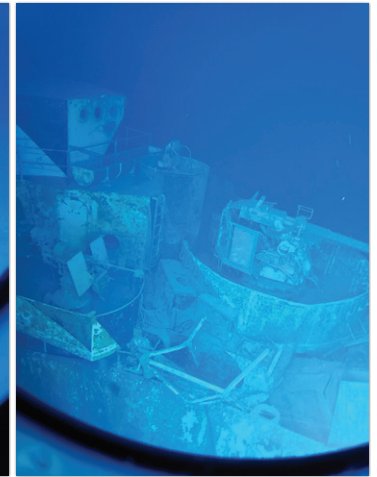
The captain's bridge of USS Samuel B. Roberts. Twin barrel of the 40 mm caliber cannon can be seen on the starboard and 20 mm cannon on the port.
