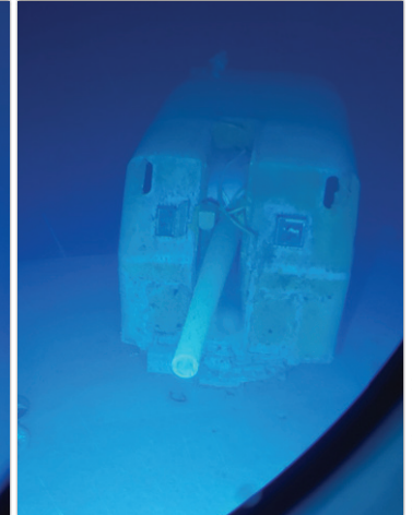
A gun turret featuring 127 mm caliber cannon on board of USS Johnston.
