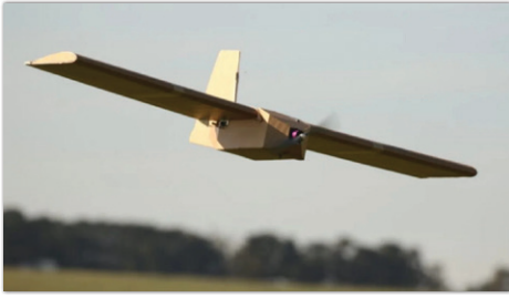
A PPDS drone from the Australian company Sypaq Corvo is made of cardboard. It can carry 5 kg of explosives.
