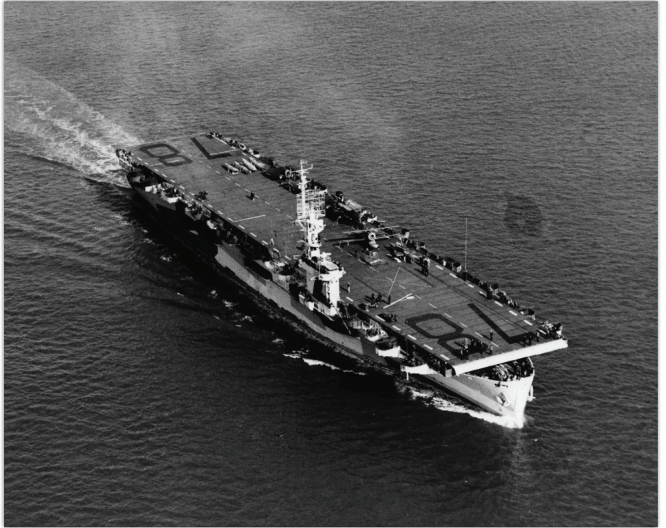
Starboard bow aerial view of Casablanca-class escort carrier USS Savo Island (CVE-78) underway. Note disassembled aircraft on the flight deck, and camouflage paint scheme.
