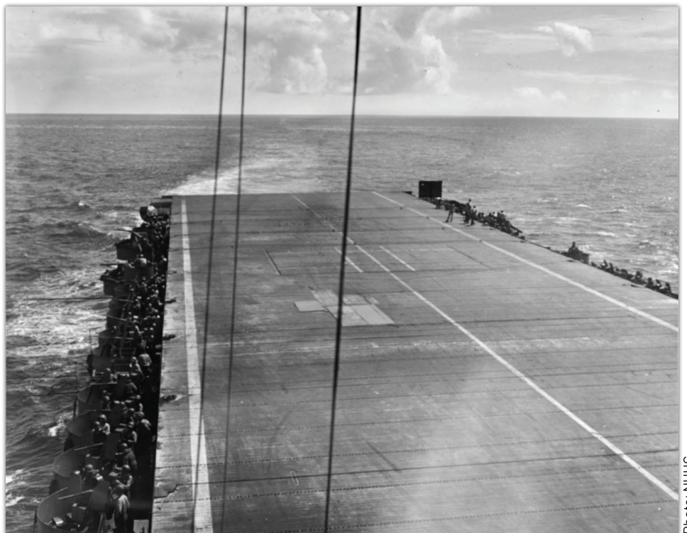
Flight deck of USS Suwannee (CVE-27) 90 minutes after a Japanese suicide plane's bomb had ripped a hole in it. Hole is patched and ship is ready to land aircraft. Note that only four wires, instead of eight, are being used. All landings were made without mishap.
