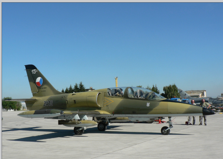
Aircraft 2415 just before taking off from the stand at the point of no return. Underslung are a pair of 150L (40 gallon) drop tanks and two live OFAB-100-110TU fragmentation bombs.
