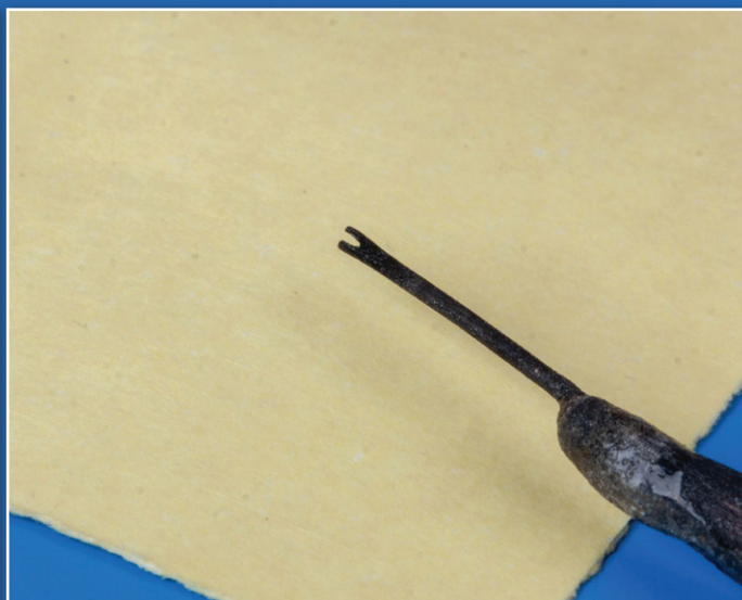
Here, you can see a close-up of the needle after modification. I use the remaining eye of the needle to scoop instant glue from the Eduard mask's base paper. The glossy surface of this paper ensures that the glue remains active for an extended period.
