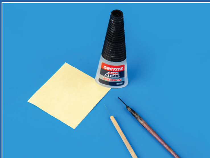
I recommend using superglue to adhere photo-etched parts. The choice of superglue can vary, and their characteristics are well-detailed in Info 04/2023. My personal preference is for extra-thin glue. To apply the glue precisely, I use a steel wire, which I've drilled into an old brush holder, and a half-flake needle, similarly drilled into a brush holder.
