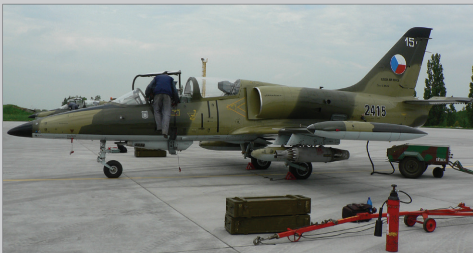
An aircraft technician removes the arming pins from the VS-1 BRI ejection seat just prior to engine start. In a few minutes, the aircraft will take off, its task will be to fire at ground targets with the GŠ-23 cannon and S-5 unguided rockets.
