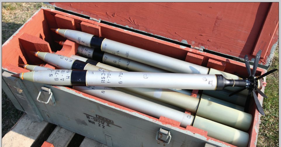
S-5 M rockets built under a Polish licence and delivered in boxes of sixteen.
