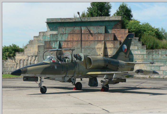
Aircraft 3903 ready for flight in front of a weathered shelter at the then Přerov aAir Base. Interestingly, it carries two full UB-16-57UMP rocket pods with 32 S-5KP missiles and two OFAB-100-110TU fragmentation bombs. Under the cockpit windscreen is a red log book.
