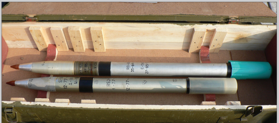
A comparison of the S-5 K and S-5 KO (top). There was an increase in the rocket motor size and the warhead of the KO, though the V-5 igniters remained the same
