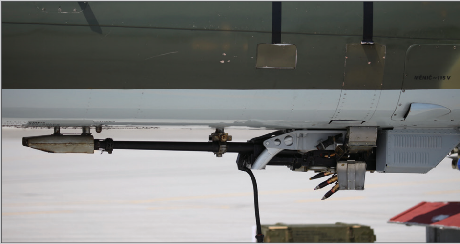
Detail view of the GŠ-23 cannon pod under the forward fuselage of the aircraft. Photo: Petr Soukup
