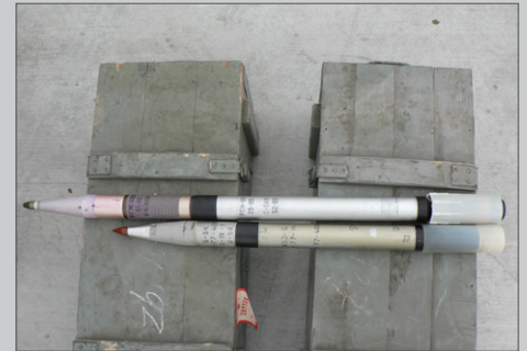
Top is the S-5 KP, below the S-5 K. The difference in the length of the rocket motor and the warhead are evident in the newer KP version. There was also a difference in the ignition system.
