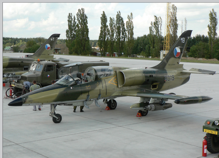
Here, the pilot is taking over aircraft 5019 from the crewchief. It carries two 40 gallon drop tanks and two full UB-16-57UMP rocket pods with 32 S-5KP unguided rockets. A special Praga V-3S SUEZ (Universal Electric Starter Source) vehicle is parked between the planes, serving as a source of electrical power during ground preparation and actual engine start-up.
