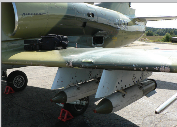
A pair of CP-100-70M practice bombs under the left wing of an L-39. The aircraft is pictured shortly after it was forced to return and land at its home field after suffering a bird strike. The damage, visible on the leading edge of the wing between the pylons, was repaired by the unit's personnel. The bird was not as lucky.
