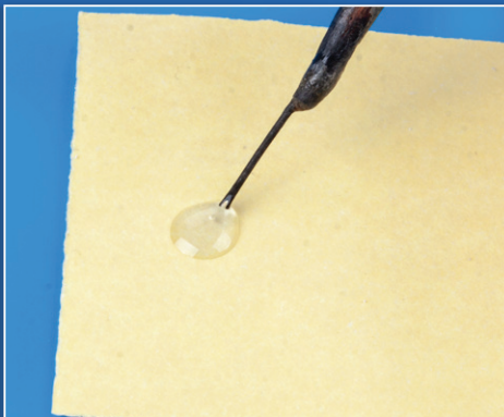
Use a tool created from a modified needle to scoop up the glue.
