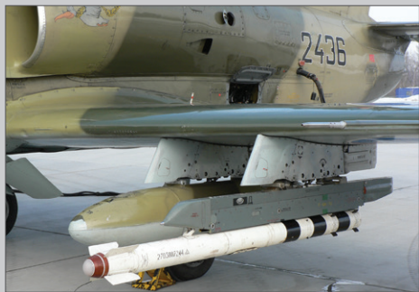
Detail view of L-39 2436 with a 150l (40 gal) drop tank and UZR-60 training round on a P-62-1M-ZA launch rail.
