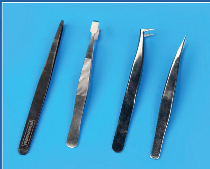
Various types of tweezers are indispensable, particularly pointed and flat-tipped tweezers. Pointed tweezers are ideal for handling and placing small parts, while flat tweezers are suitable for bending smaller components.
