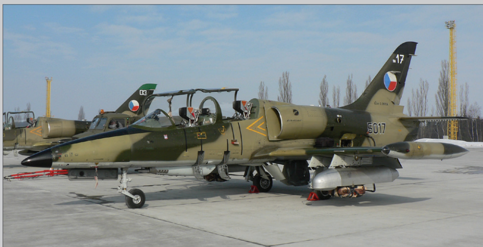
L-39 5017 carrying a special purpose container carrying a newly developed parachute readied for a test flight.
