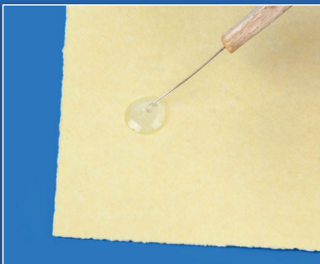
Utilize a steel wire tool to scoop up glue, which is especially useful for precise applications.
