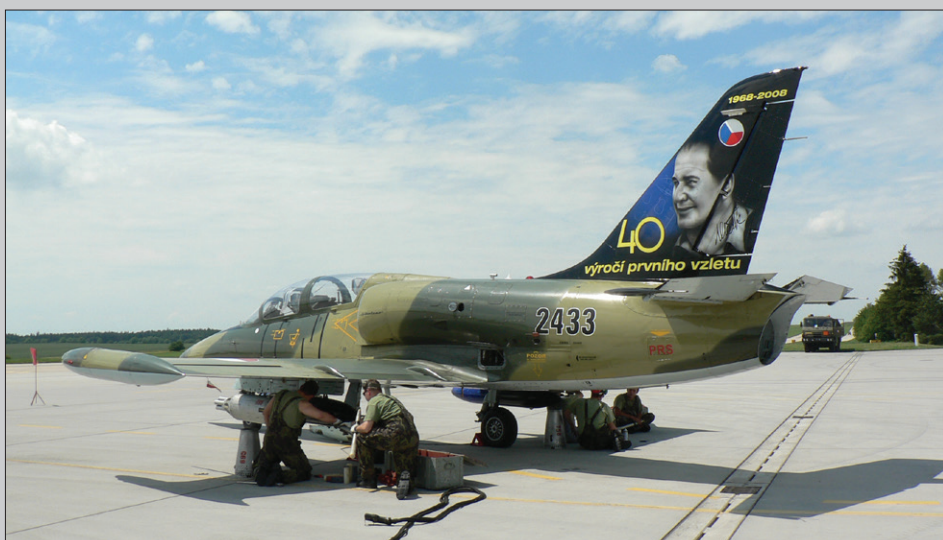
Armorers load S-5 K unguided rockets into UB-16-57 UMP rocket pods. Red flags are placed in front and behind the aircraft, external power is disconnected from the aircraft and cockpits are closed for safety reasons.
