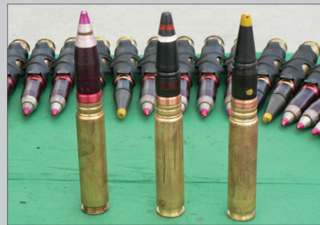
Left to right: GŠ-23 cannon pod 23mm rounds of OFZ, BZA and BZT types.
