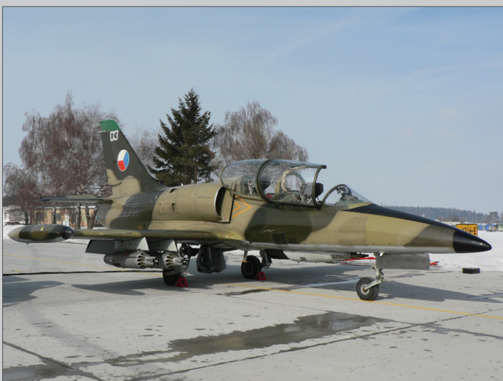
L-39ZA coded 3903 ready for flight under winter conditions at Caslav AB. The plane carries four empty UB-16-57UMP rocket pods.
