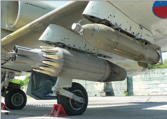
Detail of the above noted loadout. Note the weathering on the UB-16-57UMP rocket pod and the fuse delay of 0.03 seconds written down on the bomb in plain chalk.
