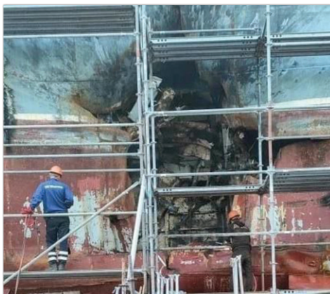
Olenegorsky Gorniyak in a dry dock showing a hole in its hull.
