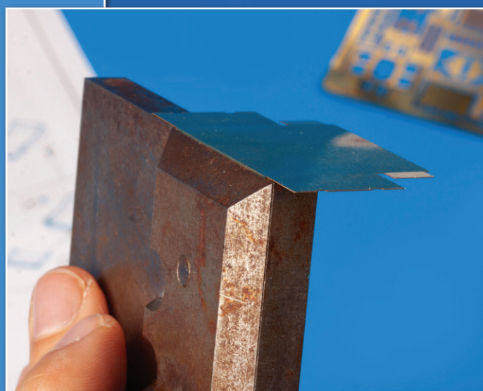
The third step involves aligning the shape of the etched detail with the bender for precise results.
