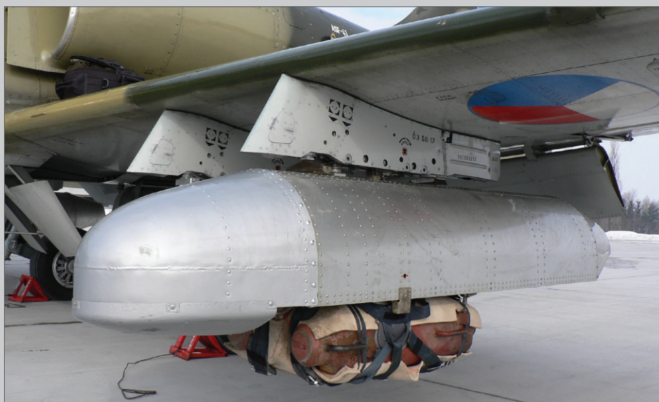
Detail shot of the pod with the parachute and weight, designed to imitate that of the human body.
