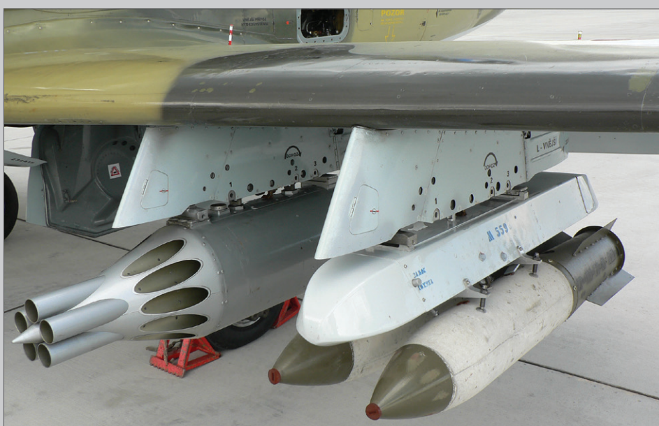
For display purposes, loaded armament could include a UB-16-57UMP rocket launcher and an L-39 M559 twin ejector rack with a pair of CP-100-70 M practice bombs.
