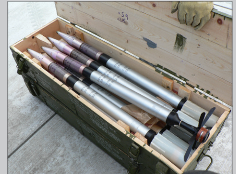
Container with eight S-5 KP rocket projectiles, one with deployed stabilization fins, which would be in flight mode. The others have their fins folded and contained in plastic caps.
