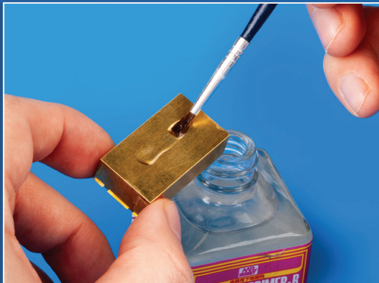
Apply Mr. Metal Primer R with a regular brush, ensuring a thin film, and allow it to dry for 15 minutes.
