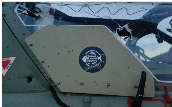
At first glance, it may not seem so, but there are 35 shrapnel hits in total in this detailed photo of the Ka-52 helicopter.
