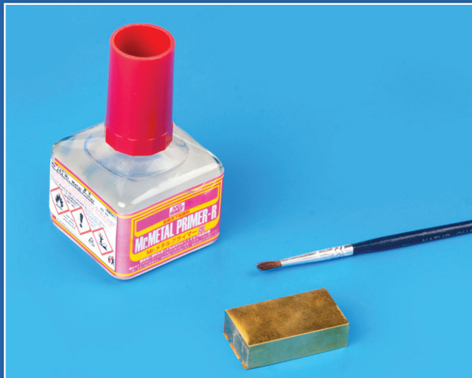
Before painting, it's advisable to recoat the already glued and bent part with Mr. Metal Primer-R.
