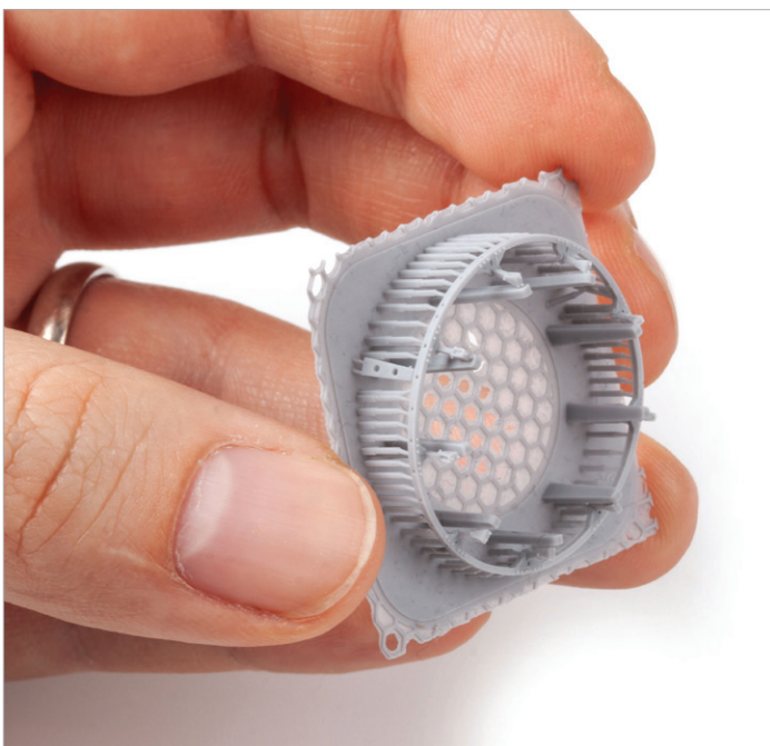
For very thin parts, use a razor saw or ultrasonic knife instead of a scalpel.
