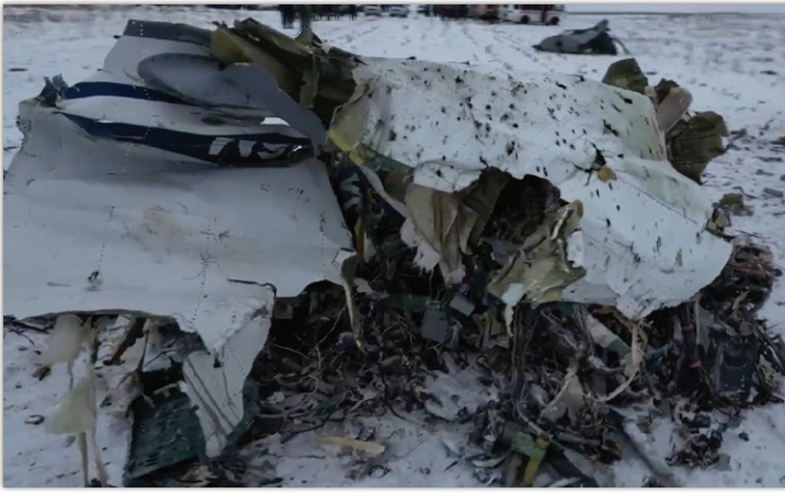
Wreckage of IL-76M shot down near the village of Jablonovo. Notice the numerous holes from shrapnel.
