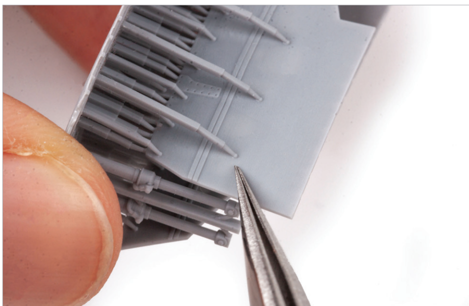
Removing Supports: Cut supports using a sharp scalpel, razor saw, or ultrasonic knife.
