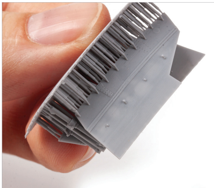
Sand the remaining supports with a fine grinder.
