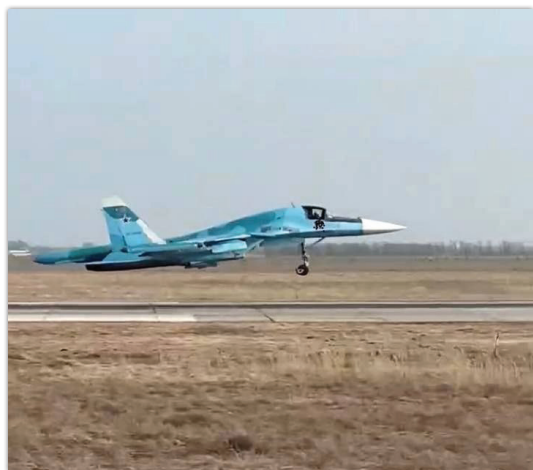
Su-34 during an emergency landing without the main landing gear. Note that the navigator is already "out."
