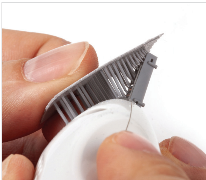
Cut through supports with the knife at a higher gear and low pressure.
