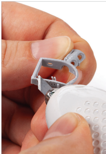
Trim any remaining residue with an ultrasonic knife.
