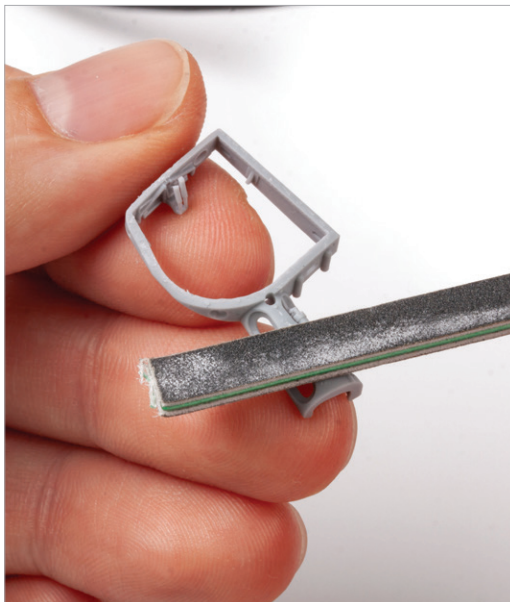
Cleaning the Part: Use a grinder to clean the entire part, opting for a coarser grinder if the side is not a visible face.
