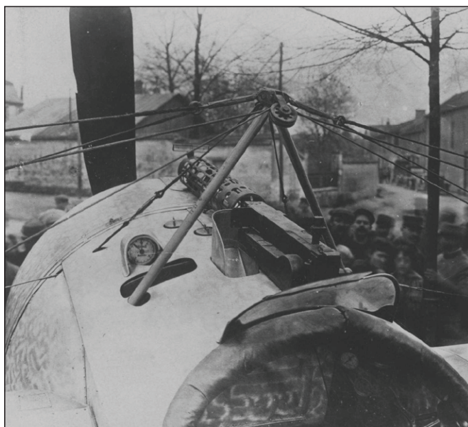
The aircraft was armed with a standard LMG08 machine gun with a wide-type sight. Photo: L'Argonnote
