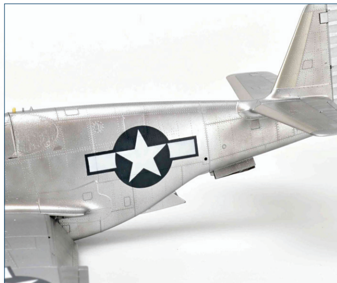
◆ I sprayed the US national insignia emblems using masks from EX1038 set.
