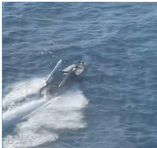
A Ukrainian naval drone equipped with an R-73 missile.
