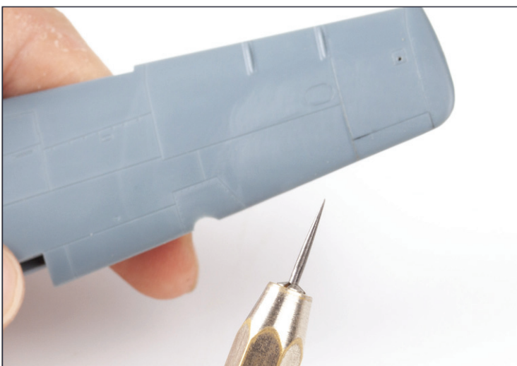
Lost rivets are restored with a phonograph needle fixed in a holder.
