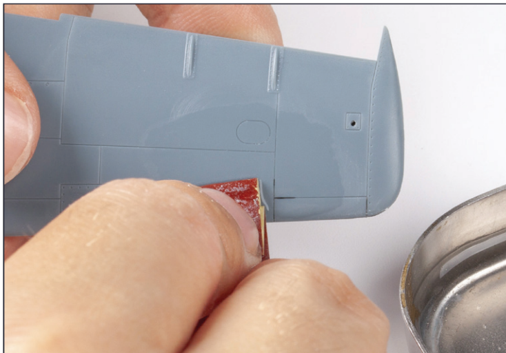
I then polish the entire area with 1500 grit sandpaper dipped in water.
