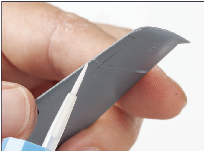
I use Mr. Cement S glue to dissolve any residual plastic dust.
