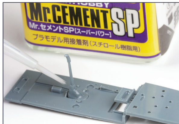
I then glue it in place using Mr. Cement SP glue. I dip the brush thoroughly into the glue, wipe the excess against the edge of the container, and then apply a sufficiently wet brush to the joint between the stick and the floor.
