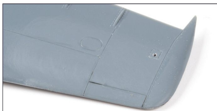
Polish and sand the joint of the wing halves. There will be no difference after applying a primer surfacer or paint.
