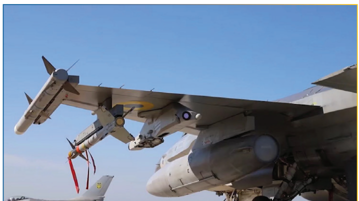
Armament of the Ukrainian F-16 – on the innermost pylon under the wing there is a fuel drop tank, followed by a pylon with the integrated PIDS+ system, and finally an AIM-9M Sidewinder missile. There is an AIM-120B missile at the wingtip.
