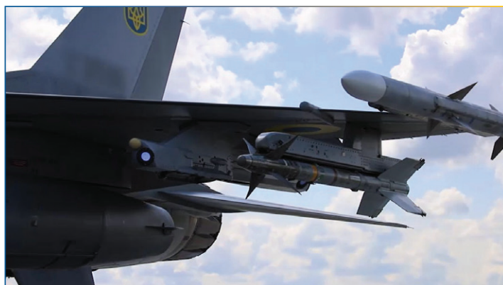
Armament of the Ukrainian F-16 – on the innermost pylon under the wing there is a fuel drop tank, followed by a pylon with the integrated PIDS+ system, and finally an AIM-9M Sidewinder missile. There is an AIM-120B missile at the wingtip.
