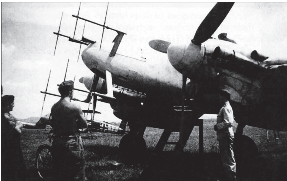
Detail on the nose of the night fighter Messerschmitt Bf 110 G from 7./NJG 6 (ZZ + GR) from the previous page. The shooting armament of this machine consisted of two MG 151 cannons instead of the classic four MG 17 and was complemented by very advanced radar technology in the form of radar FuG 220 SN-2c. Notice the flame dumpers on the exhausts.
